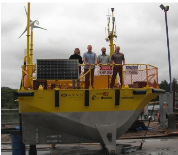
Figure 20: NNMREC's Mobile Ocean Test Berth Instrumentation Buoy, the Ocean Sentinel
