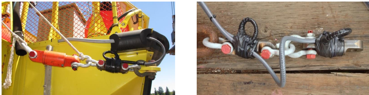
Figure 23: Ocean Sentinel mooring system with load cells integrated into each mooring line with: (left) one load cell installed on each stern mooring line where the orange swivels are used to reduce torsional forces on the load cells, and (right) two load cells used on the bow line for redundancy (not serviceable during deployment)
