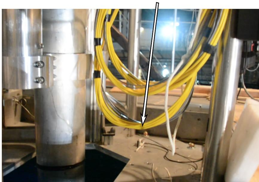
Figure 1.21: Location of triaxial accelerometer at base of PTO tower.
