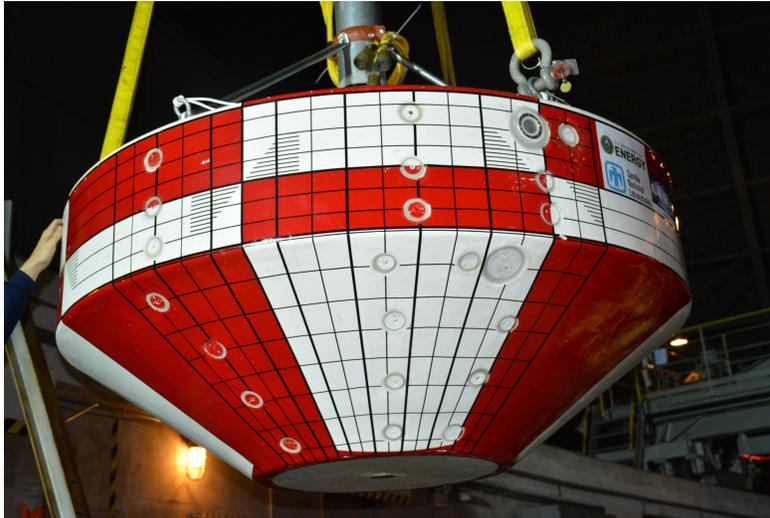
Figure 1.19: Pressure sensor ports on hull of device.
