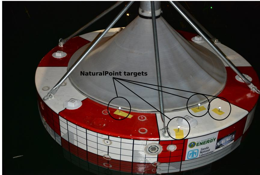
Figure 1.22: NaturalPoint optical tracking probes on float.
