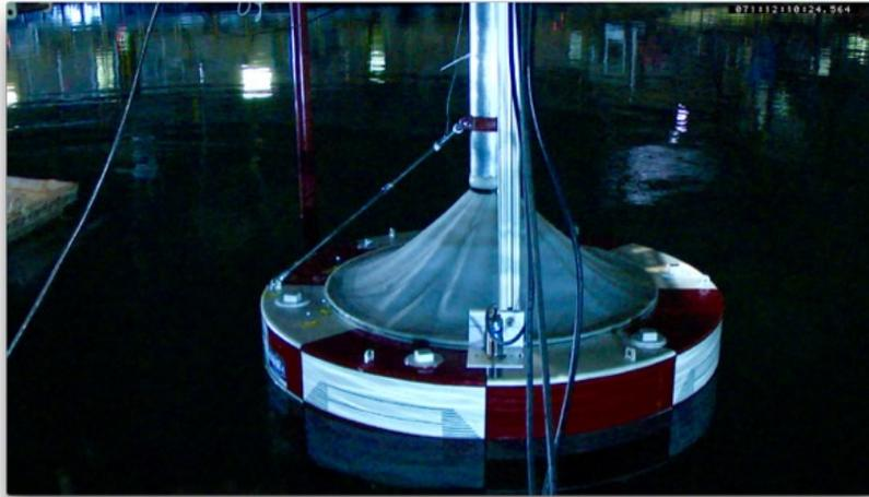
Figure 1.16: Pitch lock-out load cell installed on float.
