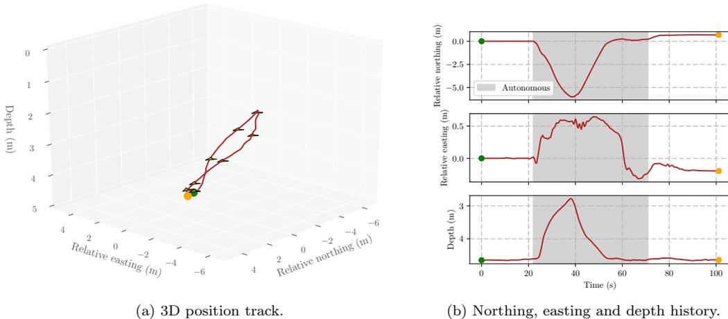
Figure 2: Navigation estimates during manipulation trial. Note that the vehicle had grasped the target at the start and end of the trajectory, so that the green (start) and yellow (end) positions of the trajectory should be approximately the same location in a fixed global frame. Heading arrows in 2a are shown in 5 s increments during autonomous motion. The grey region in 2b indicates the time during which the vehicle was under autonomous control.
