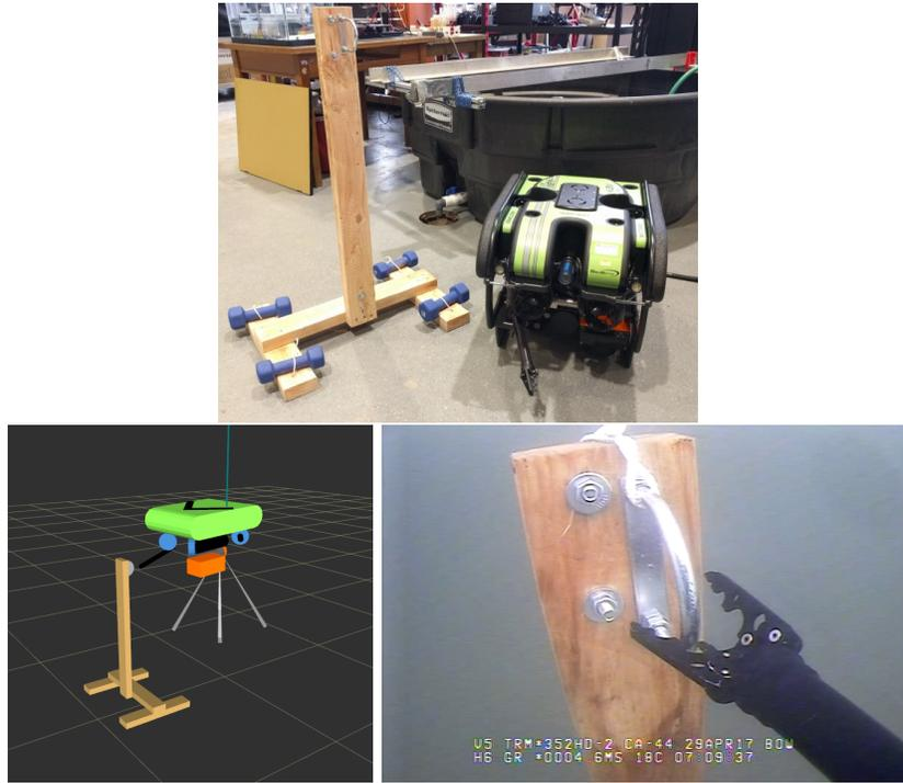
Figure 1: Photograph, onboard camera still image and ROS rviz visualization (clockwise from top left) of grasp target for shallow-water intervention trial (note that the time and date on the video overlay are incorrect, the trial was conducted on 19 June 2017).
