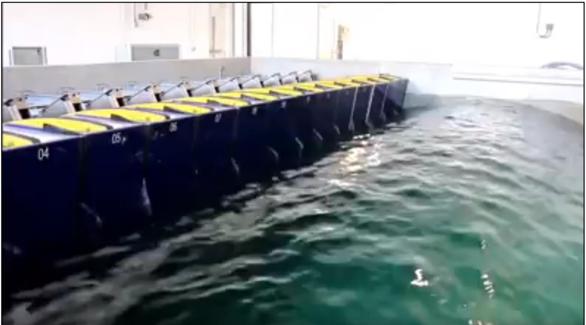
Figure 4: Wave Maker at the LIR Deep Ocean Basin
