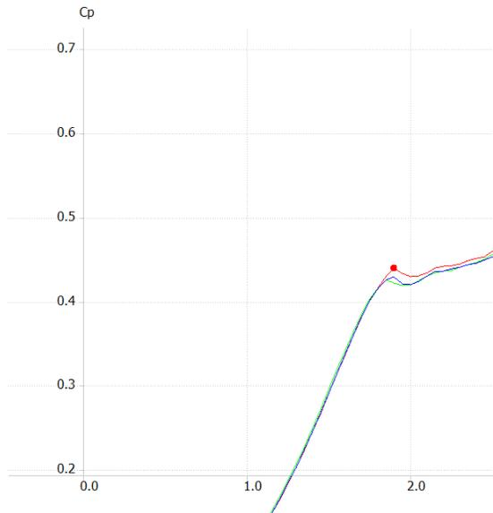
Figure 3: TidGen 1.0 baseline performance from QBlade Streamtube analysis
