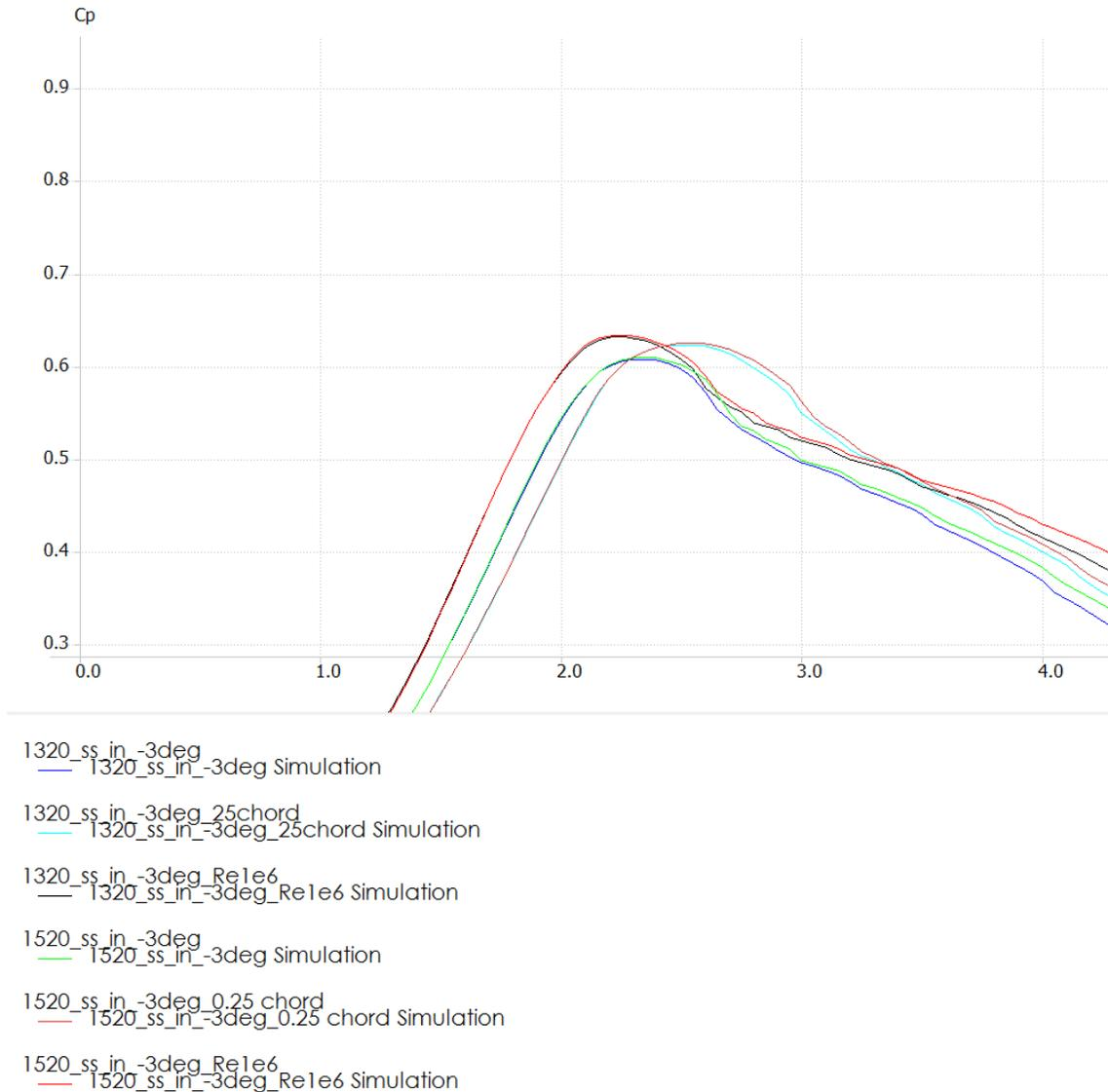
Figure 5: TidGen 2.0 study: effect of chord length on performance. Base case is 0.3m chord.
