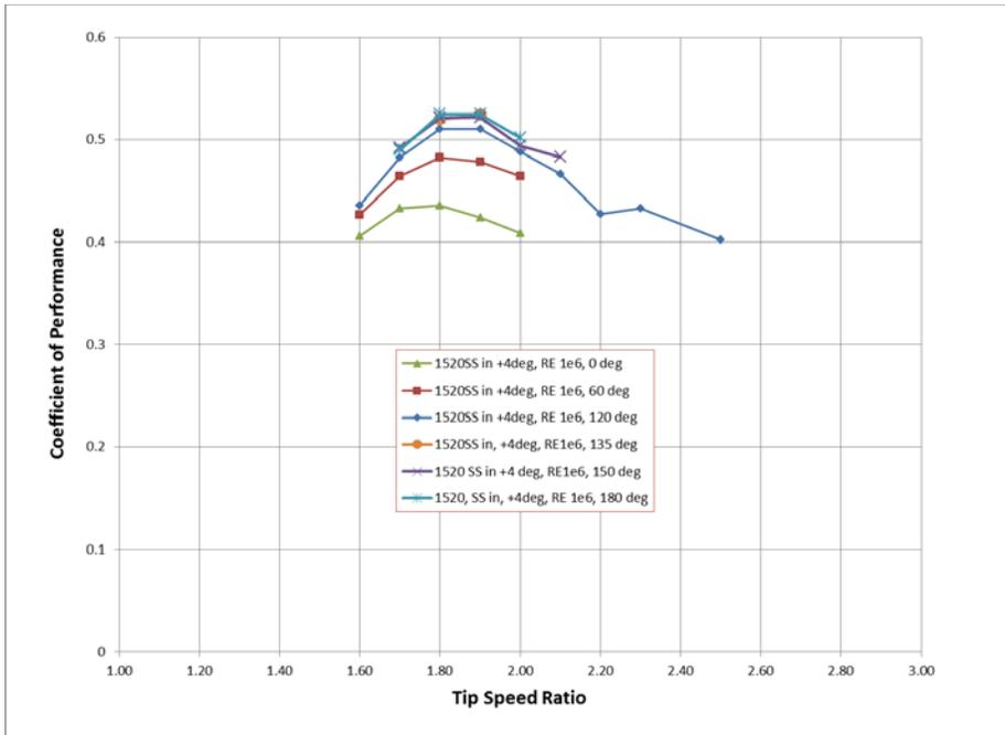
Figure 9: Effect of turbine twist on 1520 turbine performance
