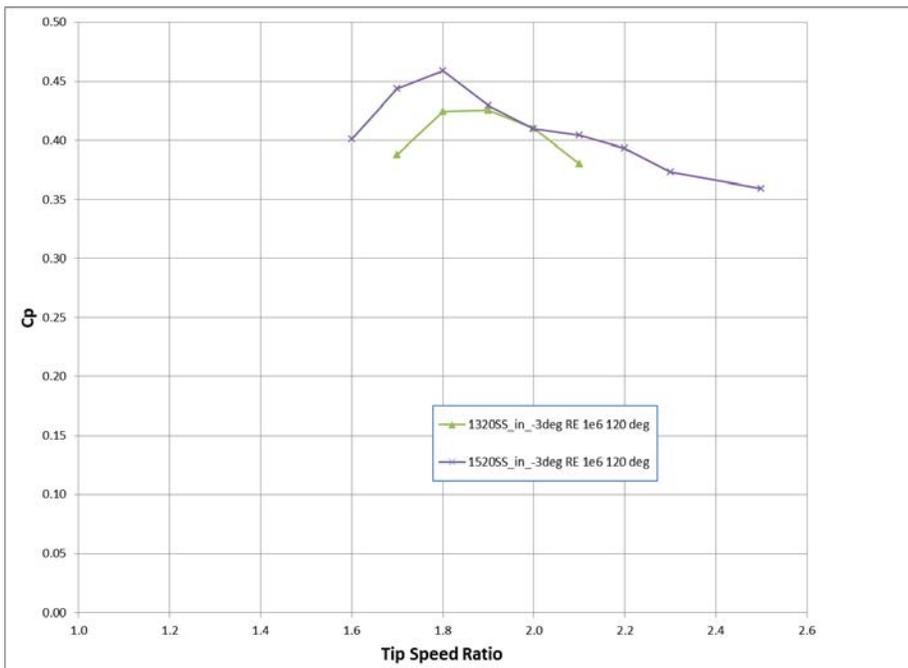
Figure 7: 1320 turbine as compared to 1520 turbine in Lifting Line analysis.
