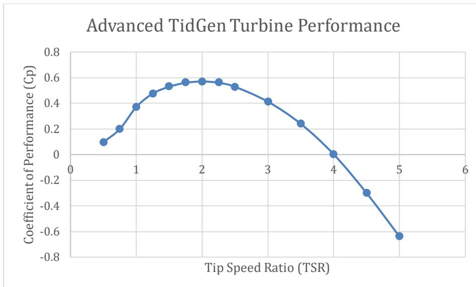
Figure 13: Advanced TidGen® 2D CFD results
