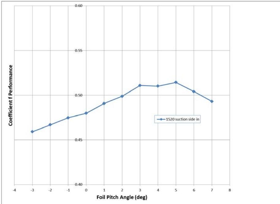
Figure 8: Effect of pitch angle on performance of 1520 turbine in Lifting Line analysis for a tip speed ratio of 1.8
