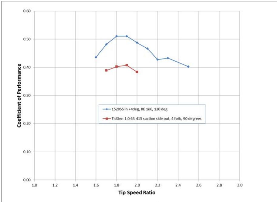
Figure 11: TidGen 2.0 compared with TidGen 1.0 Lifting Line Analysis
