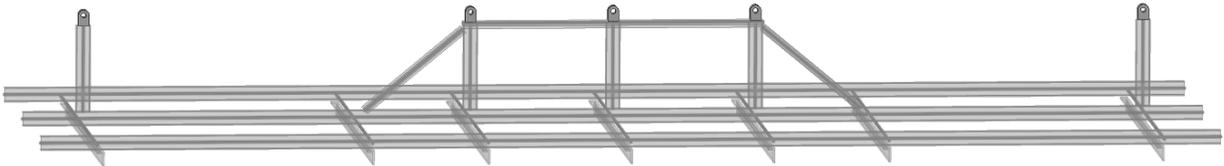
Figure 11. Steel frame and padeyes without bottom plate
