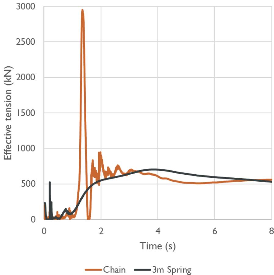
Figure 1 Mooring line suppressor comparison for snap loads
