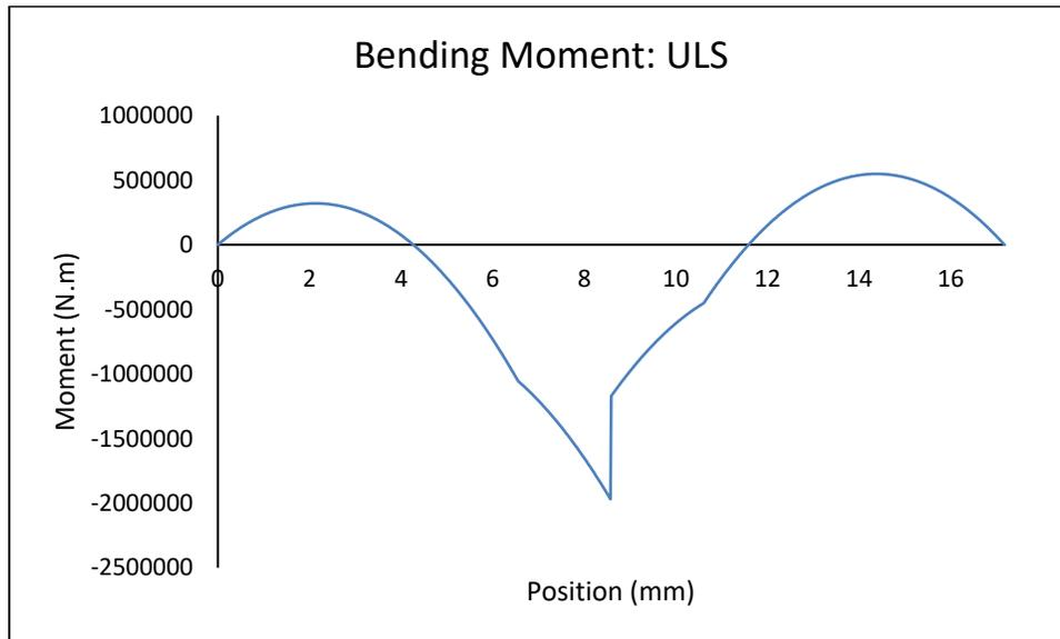
Again using simple stress-strain relationships and bending moment equations, the maximum stresses on the concrete are found to be  $6.89 \times 10^5 Pa$  in tension and  $-4.01 \times 10^5 Pa$  in compression.
