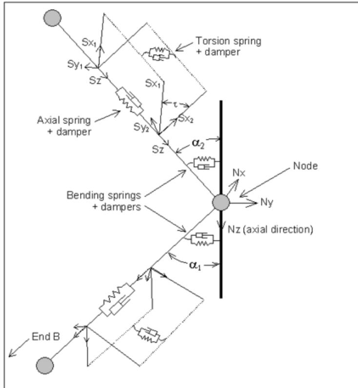
Figure 13: Representation of segment spring and damping components. Source: OrcaFlex User Manual, <https://www.orcina.com/SoftwareProducts/OrcaFlex/Documentation/Help/>.
