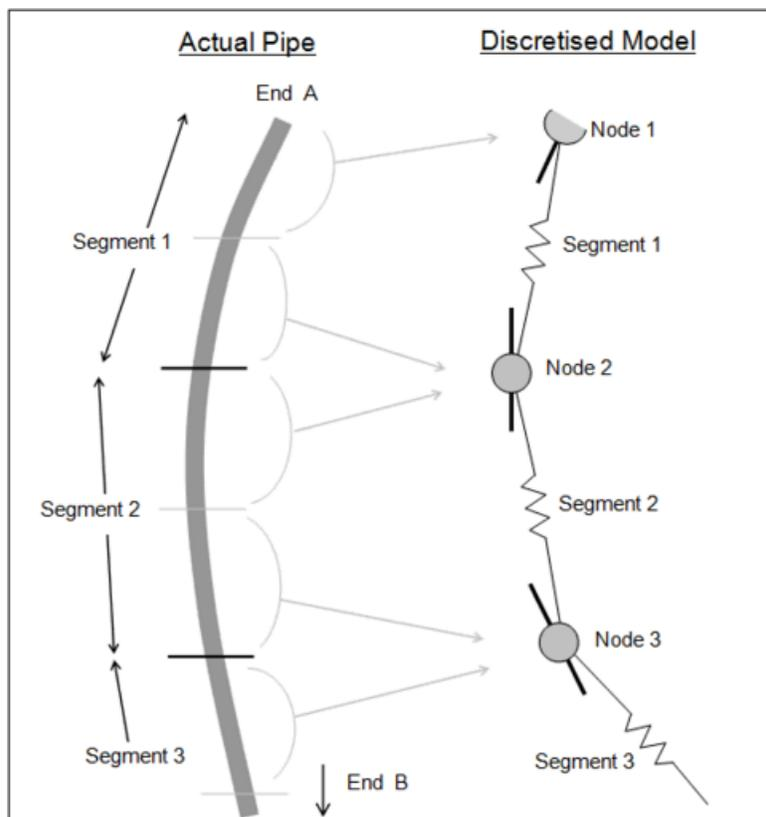
Figure 12: Typical segmentation of mooring line. Source: OrcaFlex User Manual, <https://www.orcina.com/SoftwareProducts/OrcaFlex/Documentation/Help/>.
