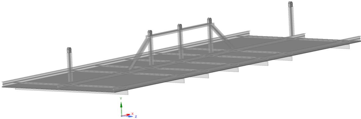
Figure 10. Steel plate, frame and padeyes embedded in concrete gravity anchor
