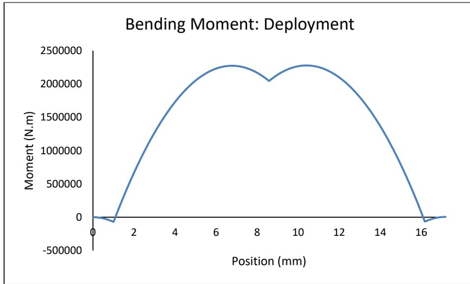
The maximum bending moment is 2,277 kN\*m. Using simple bending moment-stress relationships ( $\sigma = -\frac{My}{I}$ ), the maximum stresses in the concrete are  $8.45 \times 10^5 Pa$  in tension and  $-8.33 \times 10^5 Pa$  in compression. Assuming a representative Ultimate Strength of  $5.00 \times 10^6 Pa$  in tension and  $4.10 \times 10^7 Pa$  in compression, the stresses are well below the Ultimate Strength of the concrete.
