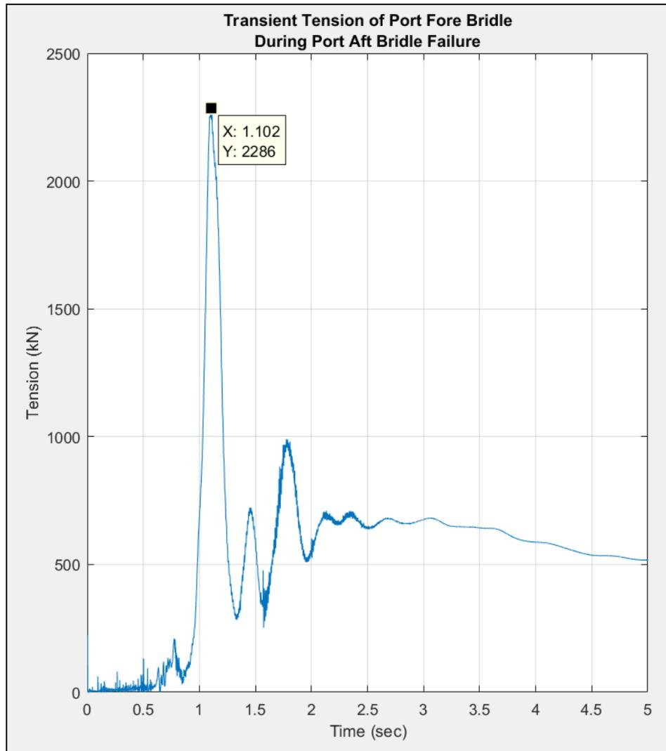
Figure 4: Simulation time history of fore bridle during aft bridle failure
