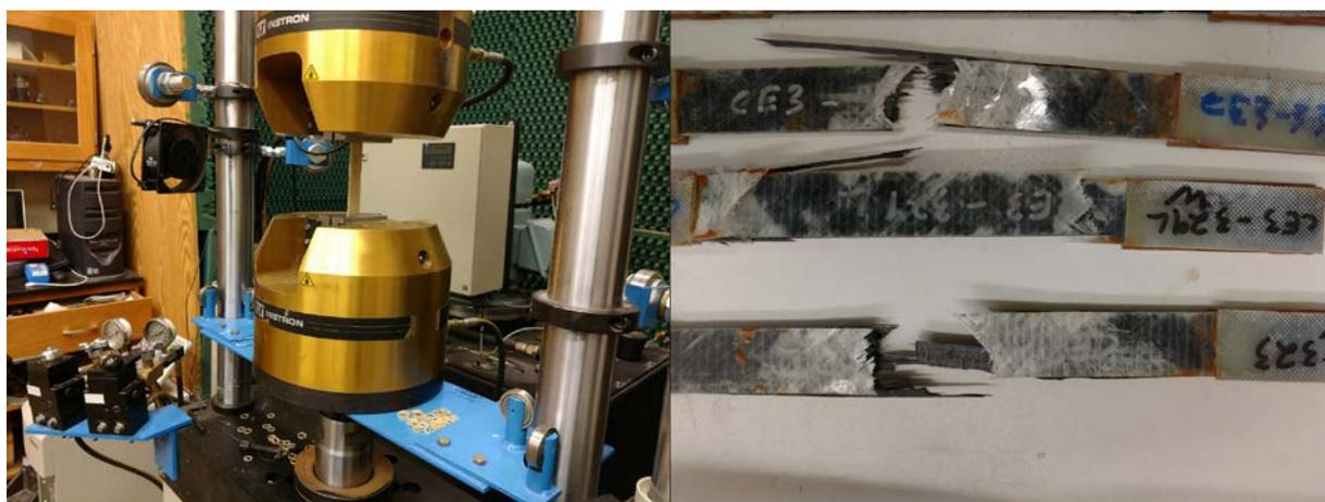
Figure 4. Coupon testing performed at Montana State University in budget period 1. Static and dynamic (fatigue) tension testing were performed as a preliminary evaluation of composite material sets in both dry and saturated (aged) states. Efforts in budget period 2 will focus on two material sets for comprehensive characterization of failure in accelerated life testing.
