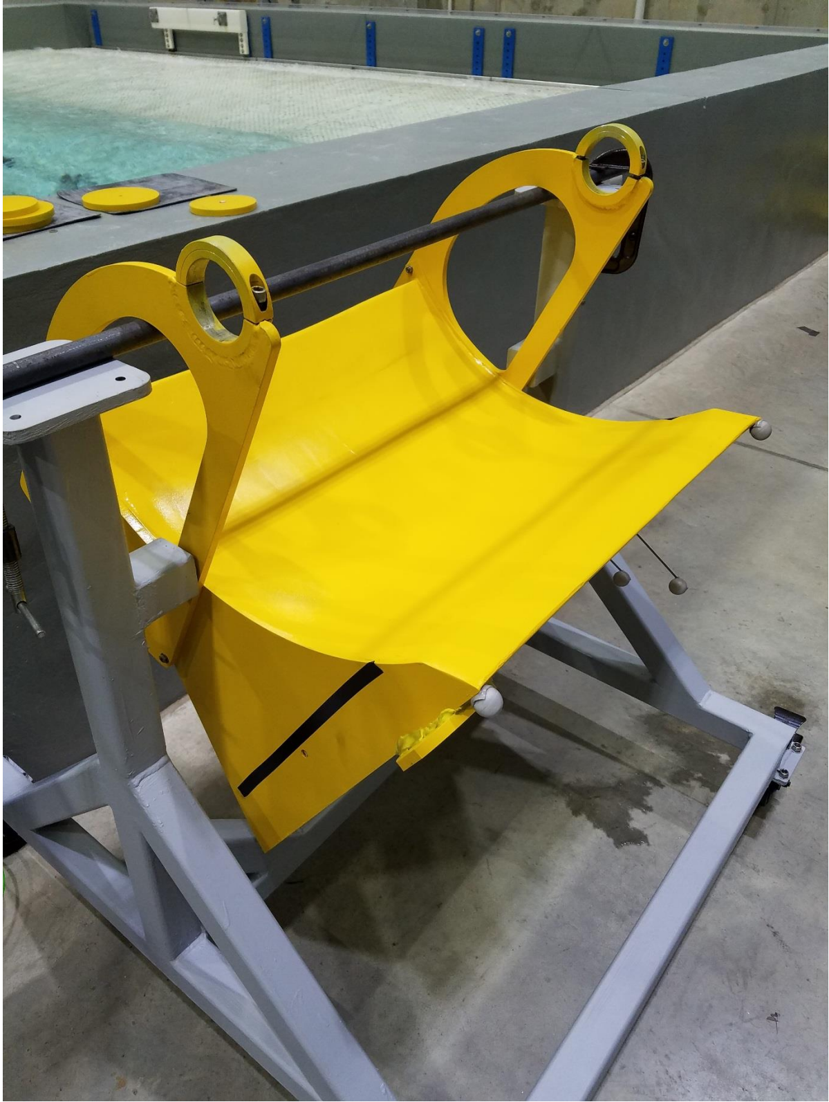
Figure 15. Float and arms on test stand
