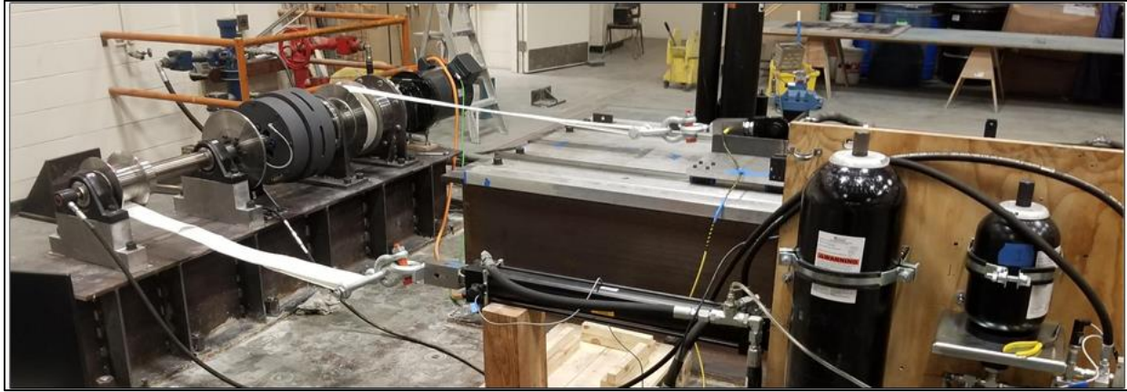
Figure 14: CalWave's PTO drivetrain assembled on the PTO bench. Here, actuation side as well as Gas-Spring side are connected to the drive shaft via PTO belts.
