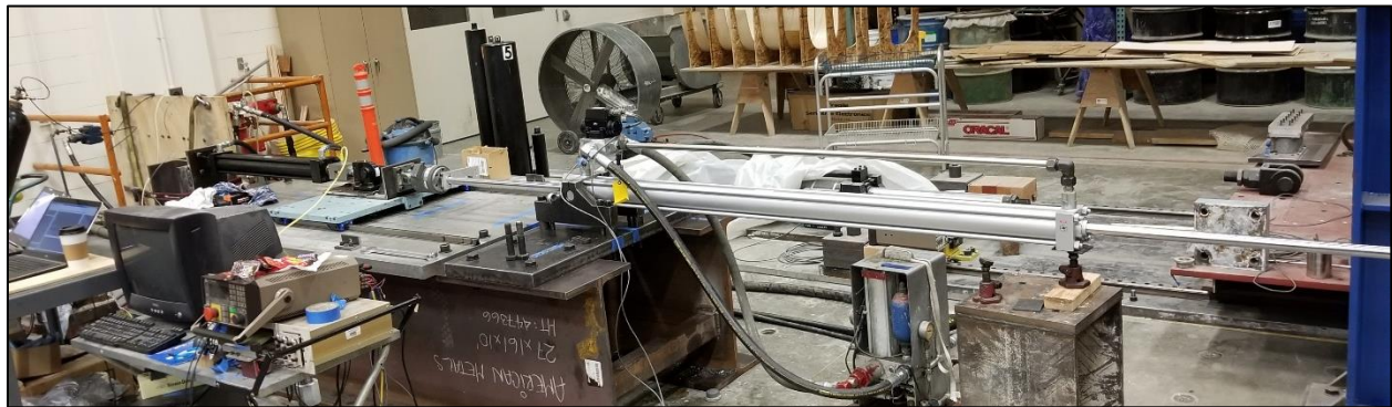
Figure 16: Gas spring test stand at the Civil Engineering department at UC Berkeley. The actuation side (right silver cylinder) tracks a controlled trajectory exciting the gas spring (left black cylinder) for characterization and assessment objectives.
