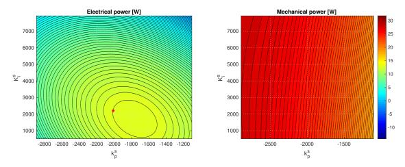
Figure 2-65. Test case 9 - Sensitivity of surge+pitch power absorption to surge control parameters. A second order 4-D polynomial has been used to fit the multidimensional surface relating the absorbed power to the controller parameters. The red mark shows the controller tuning provided by the optimization.
