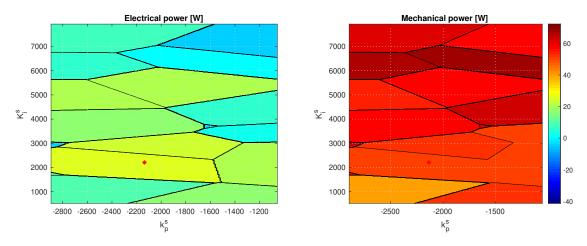
Figure 2-55. Test case 11 - Sensitivity of surge+pitch power absorption to surge control parameters.
