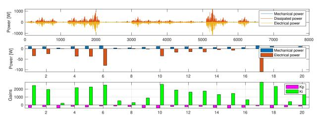
Figure 2-11. Test Case 4 - Power absorption and dissipation profiles for pitch PTO.
