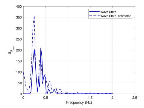
Figure 3-15. Comparison of excitation force spectra as estimated by the self-tuning controller to spectra calculated from wave height measurements for wave state CDIP139.
