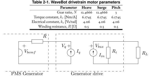
Figure 2-4. Simplified diagram of the generator and motor drive
