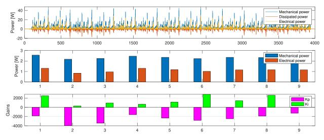
Figure 2-6. Test Case 2 - Power absorption and dissipation profiles for heave PTO.
