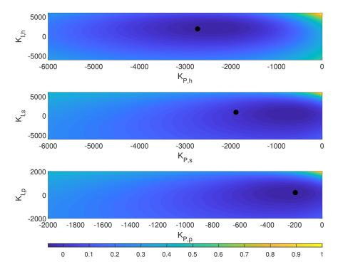
Figure 3-16. The WEC power surface as a function of gain tuning for each degree of freedom for the bi-modal wave. The color bars are normalized by the maximum absorbed power such that they are common between degrees of freedom.
