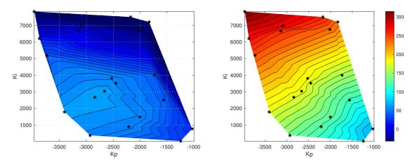
Figure 2-54. Test case 11 - Sensitivity of heave absorption to heave control parameters.
