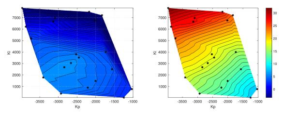
Figure 2-45. Test case 8 - Sensitivity of heave absorption to heave control parameters.
