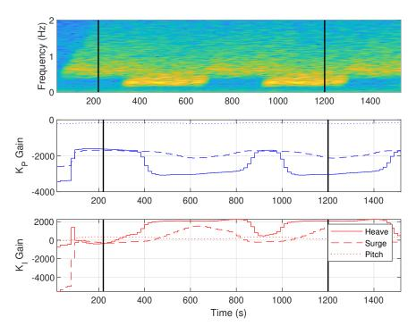
Figure 3-10. Self-tuning controller gains for changing 2A-10A wave state.
