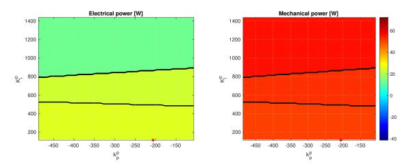
Figure 2-56. Test case 11 - Sensitivity of surge+pitch power absorption to pitch control parameters.
