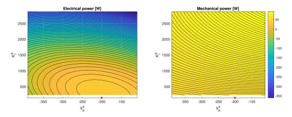
Figure 2-60. Test case 6 - Sensitivity of surge+pitch power absorption to pitch control parameters. A second order 4-D polynomial has been used to fit the multidimensional surface relating the absorbed power to the controller parameters. The red mark shows the controller tuning provided by the optimization.
