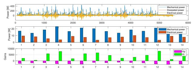
Figure 2-22. Test Case 9 - Power absorption and dissipation profiles for surge PTO.
