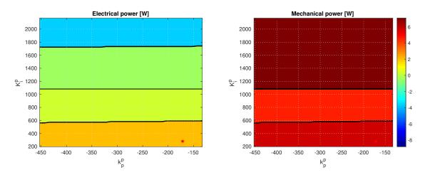
Figure 2-32. Test case 2 - Sensitivity of surge+pitch power absorption to pitch control parameters.
