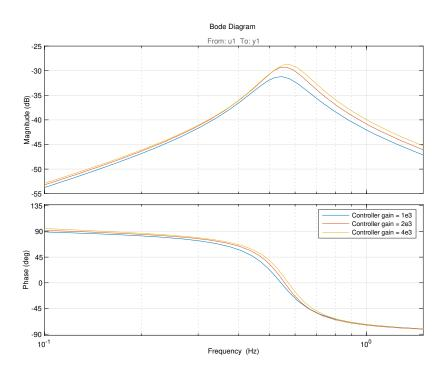
Figure 4-4. Transfer function models obtained from three wavelets of different amplitude (all with  $f_0=0.286$  Hz, s=5).
