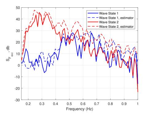
Figure 3-11. Comparison of excitation force spectra as estimated by the self-tuning controller to spectra calculated from wave height measurements for concatenated wave states 2A - 10A.
