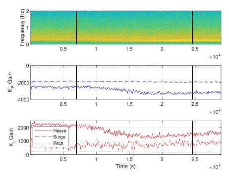
Figure 3-6. Self-tuning controller gains for the CDIP225 wave state.
