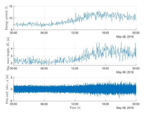
Figure 3-3. Wave time series selected for experiment (full scale).
