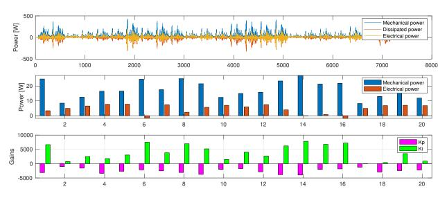
Figure 2-15. Test Case 7 - Power absorption and dissipation profiles for heave PTO.
