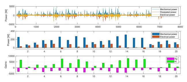
Figure 2-27. Test Case 11 -Power absorption and dissipation profiles for heave PTO.
