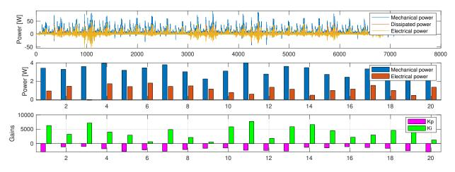
Figure 2-16. Test Case 7 - Power absorption and dissipation profiles for surge PTO.
