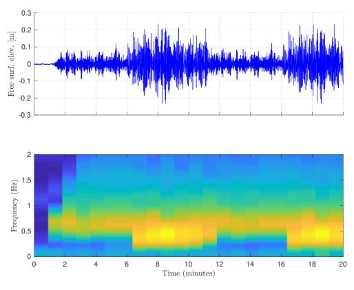
Figure 3-9. Free surface time history (top) and power spectrogram (bottom) for concatenated changing sea state (Exp 088). Sea state alternates between 2A and 6A.
