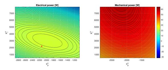
Figure 2-69. Test case 11 - Sensitivity of surge+pitch power absorption to surge control parameters. A second order 4-D polynomial has been used to fit the multidimensional surface relating the absorbed power to the controller parameters. The red mark shows the controller tuning provided by the optimization.
