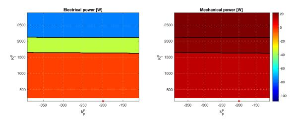
Figure 2-38. Test case 4 - Sensitivity of surge+pitch power absorption to pitch control parameters.
