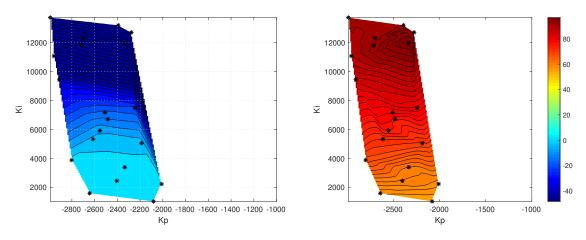
Figure 2-39. Test case 6 - Sensitivity of heave absorption to heave control parameters.
