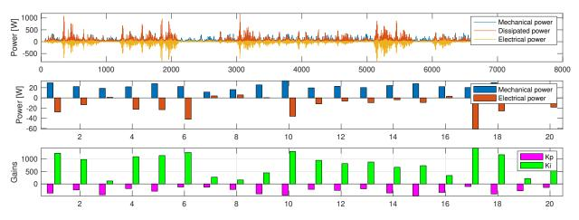
Figure 2-29. Test Case 11 -Power absorption and dissipation profiles for pitch PTO.
