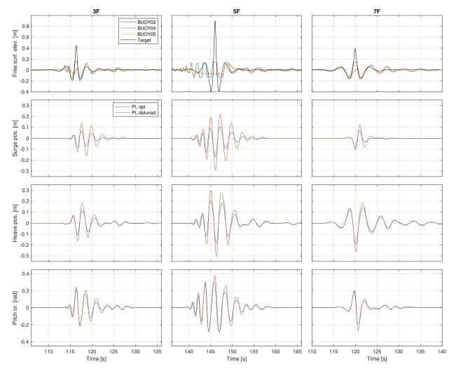
Figure 5-1. Focused wave measured calibration results and WEC responses.
