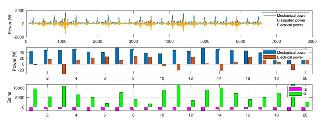
Figure 2-13. Test Case 6 - Power absorption and dissipation profiles for surge PTO.
