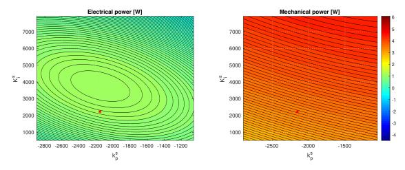
Figure 2-63. Test case 8 - Sensitivity of surge+pitch power absorption to surge control parameters. A second order 4-D polynomial has been used to fit the multidimensional surface relating the absorbed power to the controller parameters. The red mark shows the controller tuning provided by the optimization.
