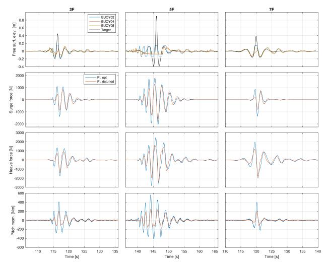
Figure 5-2. Focused wave measured calibration results and WEC PTO reactions.
