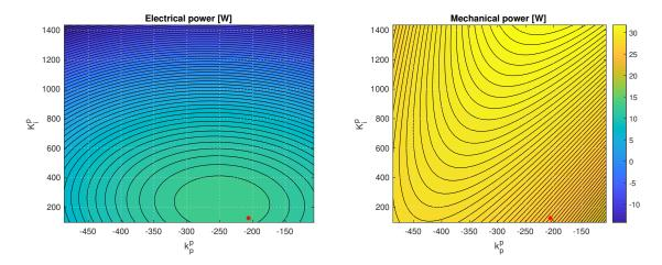
Figure 2-66. Test case 9 - Sensitivity of surge+pitch power absorption to pitch control parameters. A second order 4-D polynomial has been used to fit the multidimensional surface relating the absorbed power to the controller parameters. The red mark shows the controller tuning provided by the optimization.
