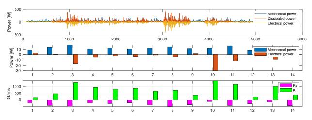
Figure 2-23. Test Case 9 - Power absorption and dissipation profiles for pitch PTO.
