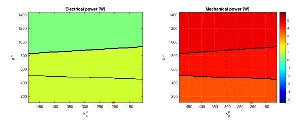
Figure 2-47. Test case 8 - Sensitivity of surge+pitch power absorption to pitch control parameters.
