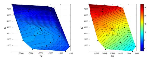
Figure 2-42. Test case 7 - Sensitivity of heave absorption to heave control parameters.
