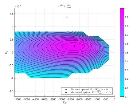
Figure D-2. Sample PI tuning results from demonstration code.
