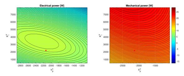
Figure 2-67. Test case 10 - Sensitivity of surge+pitch power absorption to surge control parameters. A second order 4-D polynomial has been used to fit the multidimensional surface relating the absorbed power to the controller parameters. The red mark shows the controller tuning provided by the optimization.
