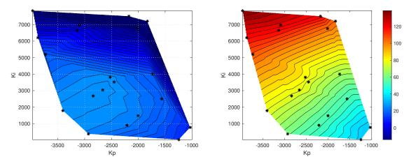
Figure 2-51. Test case 10 - Sensitivity of heave absorption to heave control parameters.
