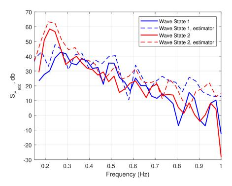
Figure 3-7. Estimates of excitation force spectra from wave height measurements (solid lines) and as estimated by the selftuning controller (dotted lines) for two contrasting wave states in the CDIP225 wave series.
