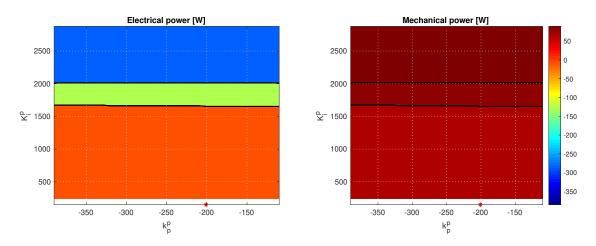
Figure 2-41. Test case 6 - Sensitivity of surge+pitch power absorption to pitch control parameters.
