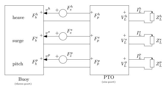
Figure 2-2. Multi-Port representation on the WaveBot
