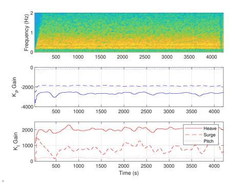
Figure 3-14. Self-tuning controller gains for bimodal CDIP139 sea state.
