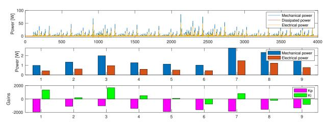
Figure 2-7. Test Case 2 - Power absorption and dissipation profiles for surge PTO.
