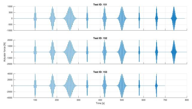
Figure 4-1. Heave only wavelet applied force.
