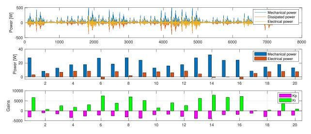
Figure 2-18. Test Case 8 - Power absorption and dissipation profiles for heave PTO.
