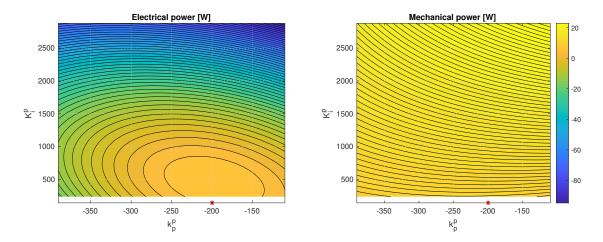
Figure 2-58. Test case 4 - Sensitivity of surge+pitch power absorption to pitch control parameters. A second order 4-D polynomial has been used to fit the multidimensional surface relating the absorbed power to the controller parameters. The red mark shows the controller tuning provided by the optimization.
