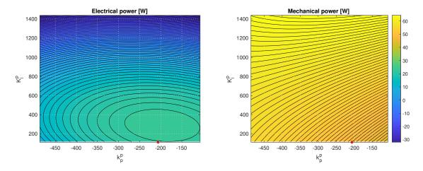
Figure 2-70. Test case 11 - Sensitivity of surge+pitch power absorption to pitch control parameters. A second order 4-D polynomial has been used to fit the multidimensional surface relating the absorbed power to the controller parameters. The red mark shows the controller tuning provided by the optimization.
