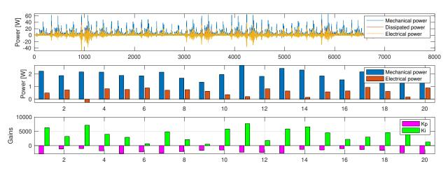
Figure 2-19. Test Case 8 - Power absorption and dissipation profiles for surge PTO.
