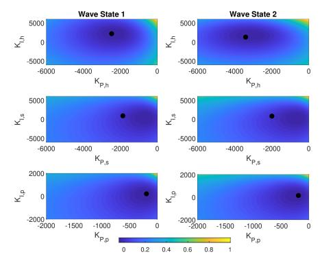
Figure 3-8. The WEC power surface as a function of gain tuning for each degree of freedom and wave state for the CDIP225 wave. The color bars are normalized by the maximum absorbed power such that they are common between degrees of freedom.
