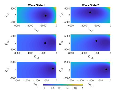
Figure 3-12. The WEC power surface as a function of gain tuning for each degree of freedom and wave state for the 2A-10A concatenated wave. The color bars are normalized by the maximum absorbed power such that they are common between degrees of freedom.
