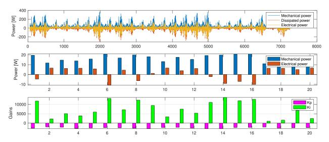
Figure 2-9. Test Case 4 - Power absorption and dissipation profiles for heave PTO.
