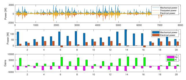
Figure 2-24. Test Case 10 -Power absorption and dissipation profiles for heave PTO.
