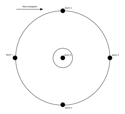
Figure 1-3. Layout of wave probes at WEC location. The probes BUOY02, BUOY04, and BUOY05 are all in line with the center of the WEC with respect to the wave front. BUOY05 is located close to the center of the WEC.
