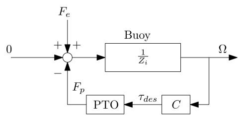
Figure 2-5. WaveBot controller structure block diagram
