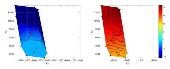
Figure 2-36. Test case 4 - Sensitivity of heave absorption to heave control parameters.
