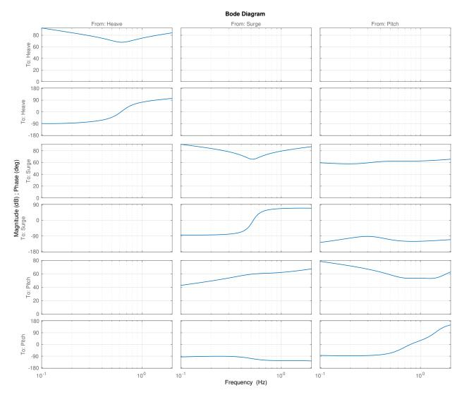
Figure 2-3. Multi-input, multi-output (MIMO) impedance system for WaveBot.
