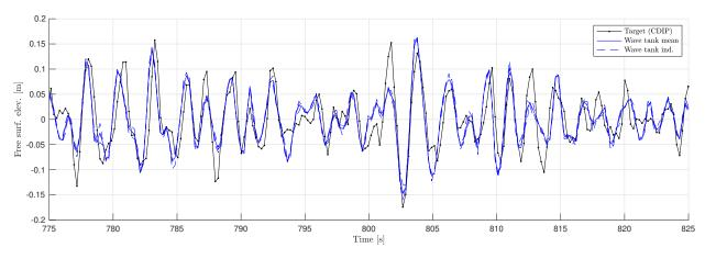
Figure 3-4. Segment of time history for CDIP225  $\lambda = 1/12$  wave calibration (Exp 093).
