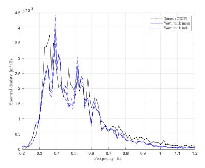
Figure 3-5. Spectral energy density comparison for CDIP225  $\lambda=1/12$  wave calibration (Exp 093).
