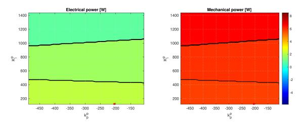
Figure 2-44. Test case 7 - Sensitivity of surge+pitch power absorption to pitch control parameters.
