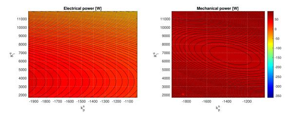
Figure 2-59. Test case 6 - Sensitivity of surge+pitch power absorption to surge control parameters. A second order 4-D polynomial has been used to fit the multidimensional surface relating the absorbed power to the controller parameters. The red mark shows the controller tuning provided by the optimization.
