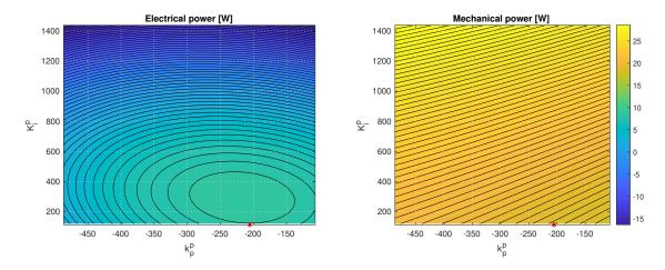
Figure 2-68. Test case 10 - Sensitivity of surge+pitch power absorption to pitch control parameters. A second order 4-D polynomial has been used to fit the multidimensional surface relating the absorbed power to the controller parameters. The red mark shows the controller tuning provided by the optimization.
