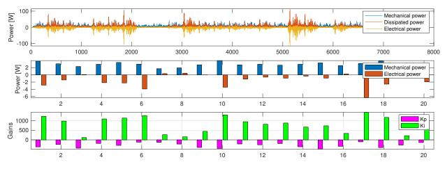
Figure 2-20. Test Case 8 - Power absorption and dissipation profiles for pitch PTO.
