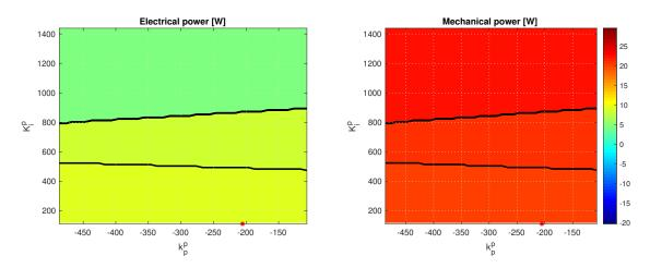
Figure 2-53. Test case 10 - Sensitivity of surge+pitch power absorption to pitch control parameters.
