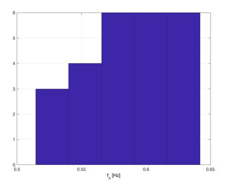
Figure 4-3. Distribution of natural frequencies from transfer function models obtained from 26 wavelets.
