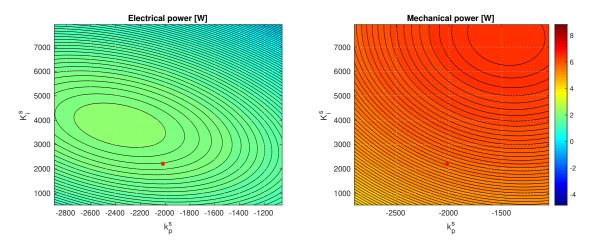
Figure 2-61. Test case 7 - Sensitivity of surge+pitch power absorption to surge control parameters. A second order 4-D polynomial has been used to fit the multidimensional surface relating the absorbed power to the controller parameters. The red mark shows the controller tuning provided by the optimization.
