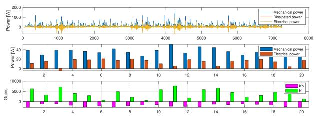
Figure 2-28. Test Case 11 -Power absorption and dissipation profiles for surge PTO.
