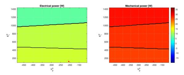
Figure 2-50. Test case 9 - Sensitivity of surge+pitch power absorption to pitch control parameters.
