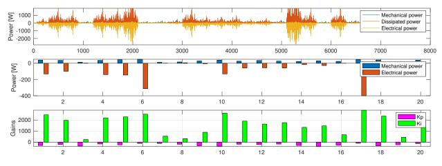
Figure 2-14. Test Case 6 - Power absorption and dissipation profiles for pitch PTO.
