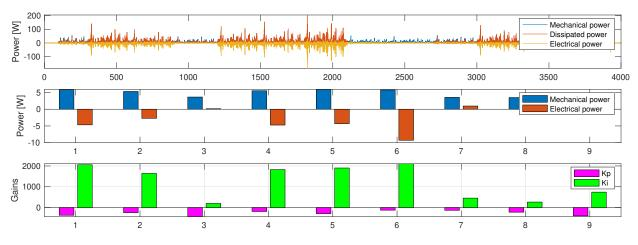
Figure 2-8. Test Case 2 - Power absorption and dissipation profiles for pitch PTO.
