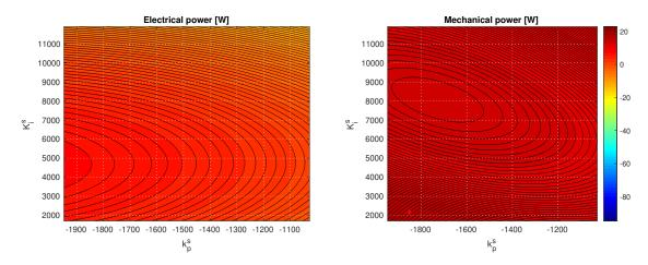
Figure 2-57. Test case 4 - Sensitivity of surge+pitch power absorption to surge control parameters. A second order 4-D polynomial has been used to fit the multidimensional surface relating the absorbed power to the controller parameters. The red mark shows the controller tuning provided by the optimization.
