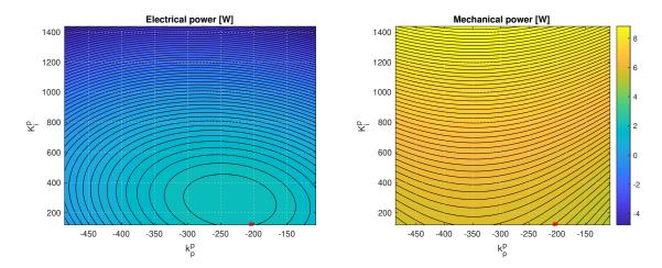
Figure 2-62. Test case 7 - Sensitivity of surge+pitch power absorption to pitch control parameters. A second order 4-D polynomial has been used to fit the multidimensional surface relating the absorbed power to the controller parameters. The red mark shows the controller tuning provided by the optimization.
