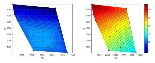
Figure 2-48. Test case 9 - Sensitivity of heave absorption to heave control parameters.
