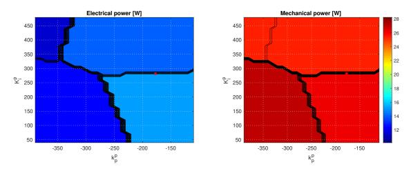
Figure 2-35. Test case 13 - Sensitivity of surge+pitch power absorption to pitch control parameters.
