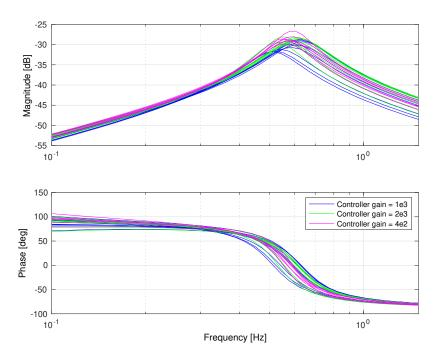
Figure 4-2. Transfer function models obtained from 26 wavelets. Controller gains are shown by blue: 1e3, green: 2e3, magenta: 4e3.
