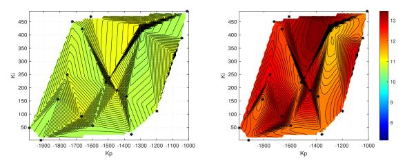
Figure 2-33. Test case 13 - Sensitivity of heave absorption to heave control parameters.
