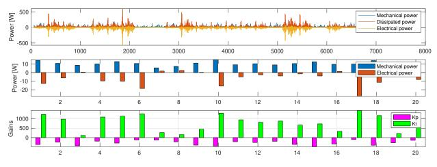
Figure 2-26. Test Case 10 -Power absorption and dissipation profiles for pitch PTO.
