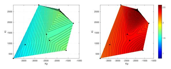
Figure 2-30. Test case 2 - Sensitivity of heave absorption to heave control parameters.
