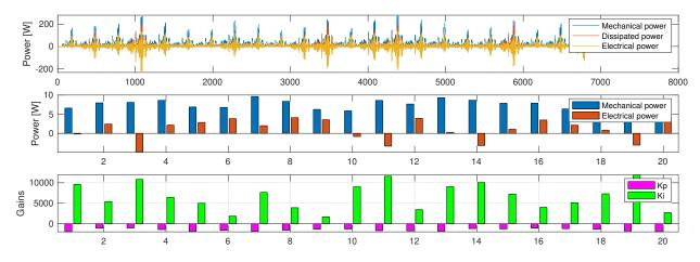
Figure 2-10. Test Case 4 - Power absorption and dissipation profiles for surge PTO.
