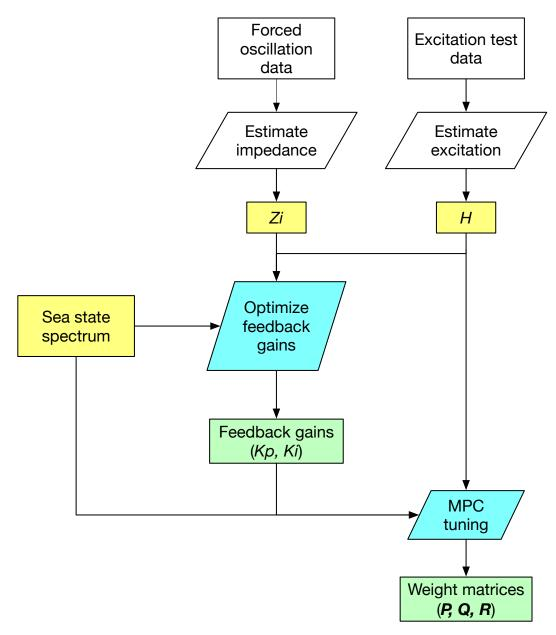
Figure D-1. Control design work-flow for demonstration code.
