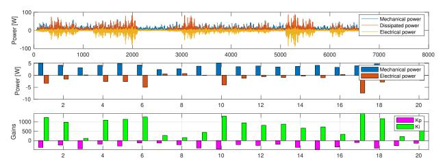
Figure 2-17. Test Case 7 - Power absorption and dissipation profiles for pitch PTO.
