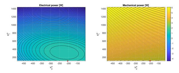
Figure 2-64. Test case 8 - Sensitivity of surge+pitch power absorption to pitch control parameters. A second order 4-D polynomial has been used to fit the multidimensional surface relating the absorbed power to the controller parameters. The red mark shows the controller tuning provided by the optimization.
