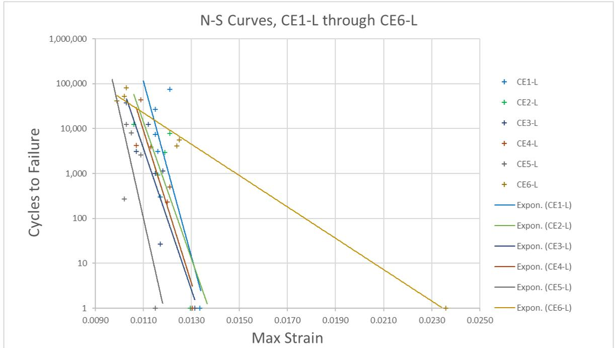
FIGURE 5: CYCLES TO FAILURE VS. STRAIN
