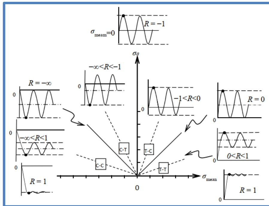
FIGURE 1: STRESS RATIO RANGES ON A  $\sigma_a - \sigma_{mean}$  DIAGRAM FOR THE LOADING TYPES: T-T, T-C, C-T, AND C-C.
