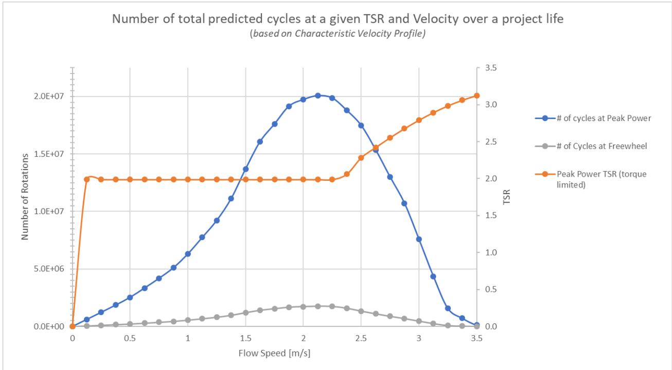
FIGURE 6, NUMBER OF TURBINE ROTATIONS VERSUS FLOW SPEED
