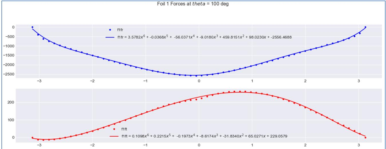
FIGURE 2, RADIAL LOADS (TOP) AND TANGENTIAL LOADS (BOTTOM) FOR FOIL 1 AT 100 DEGREES OF ROTATION
