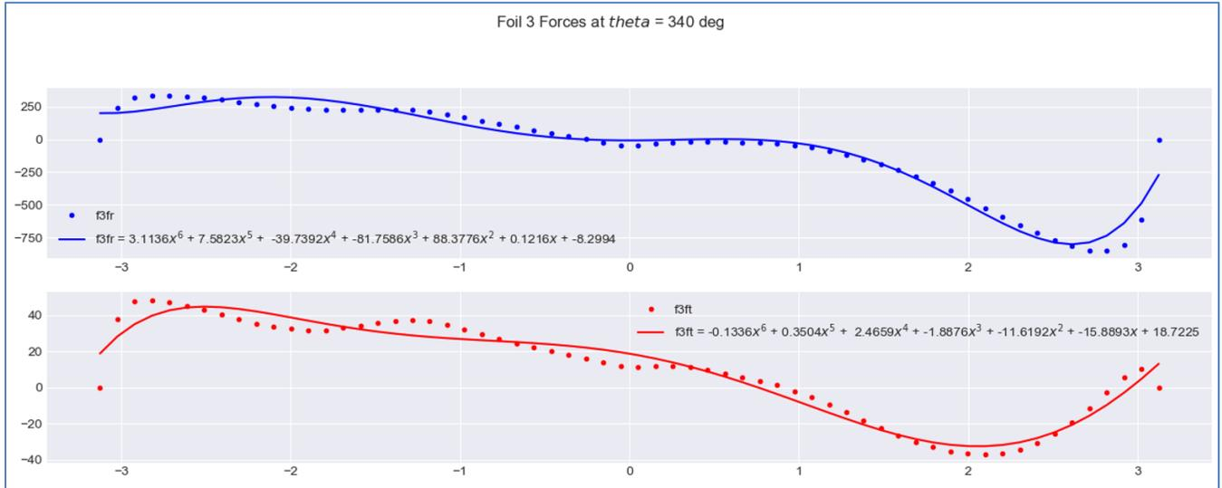
FIGURE 4, RADIAL LOADS (TOP) AND TANGENTIAL LOADS (BOTTOM) FOR FOIL 3 AT 340 DEGREES OF ROTATION
