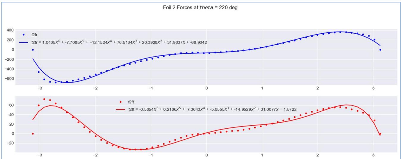
FIGURE 3, RADIAL LOADS (TOP) AND TANGENTIAL LOADS (BOTTOM) FOR FOIL 2 AT 220 DEGREES OF ROTATION
