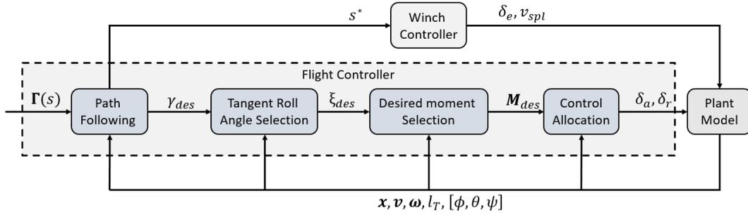
Fig. 2. Block diagram of the control system where  $\mathbf{x}$  is the position vector,  $\mathbf{v}$  is the velocity vector,  $\boldsymbol{\omega}$  is the kite angular velocity vector,  $l_T$  is the un-spooled tether length, and  $[\phi, \theta, \psi]$  is the vector of Euler angles (roll, pitch and yaw respectively).
