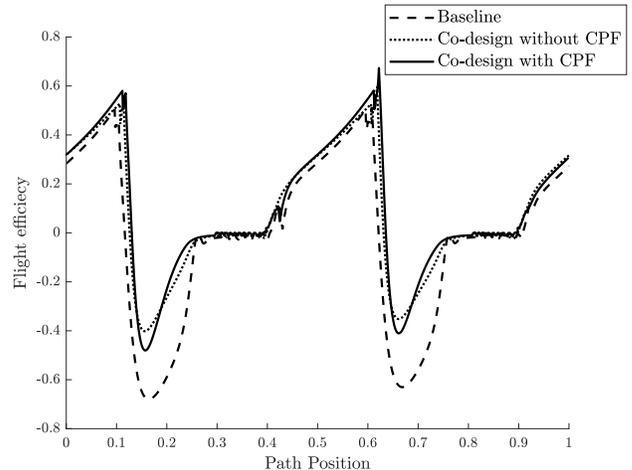
Fig. 7. Results comparing the flight efficiency  $\eta$  of the baseline, optimized kites - with and without the CPF. The results show the kites' flight efficiencies over a single lap in a constant flow regime, with flow speed of 1.5 m/s.
