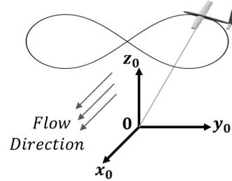
Fig. 1. The ocean kite flying in a figure-8 path, with the inertial frame of reference at the winch shown as 0 and the flow of the current being along the  $x_0$ .
