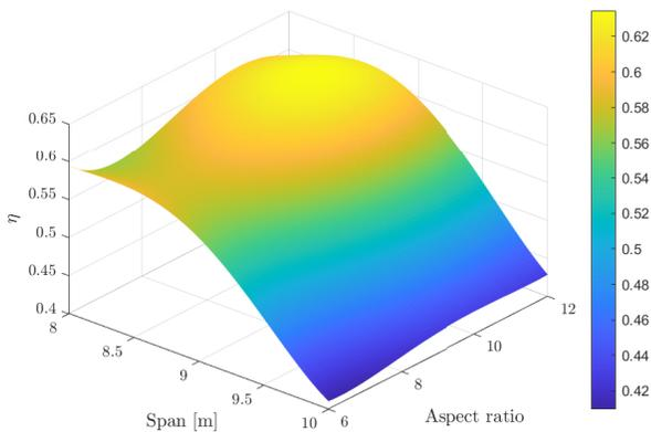
Fig. 5. Results of sensitivity analysis: A flight efficiency map that relates the dynamically simulated power generated  $P_{\text{gen}}$  to the theoretically calculated and optimized power  $P_{\text{ideal}}$  calculated in (12).
