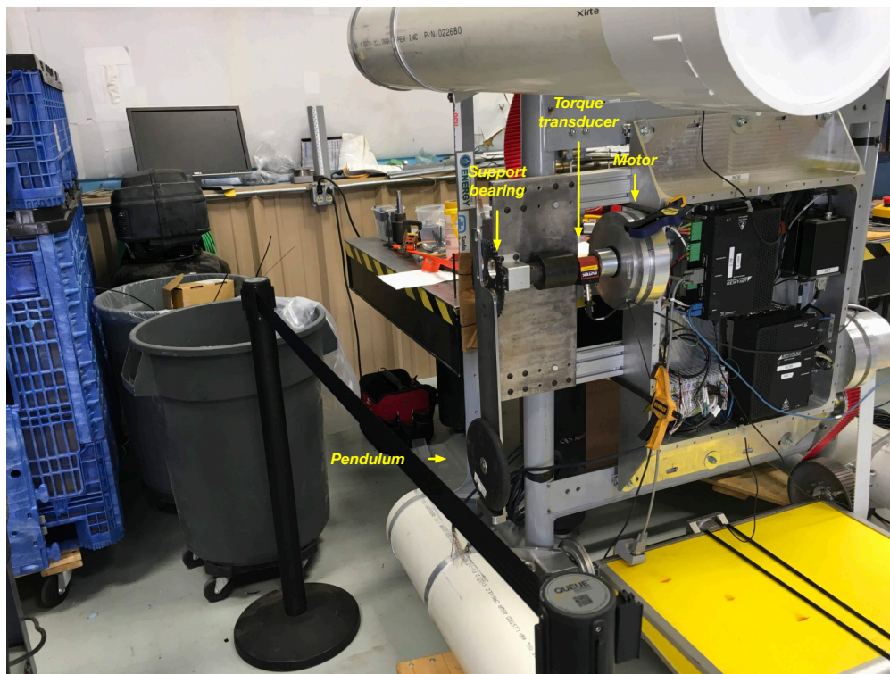
Figure E-2 Bench test set up for pendulum tests.
