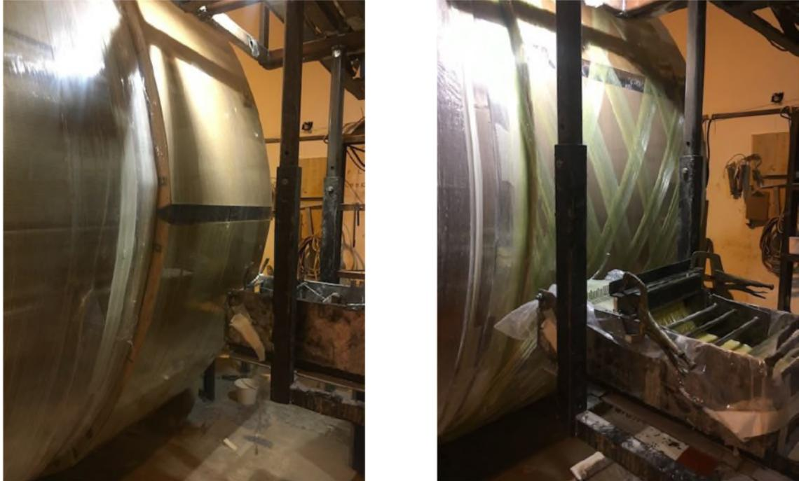
Figure 3 – Filament winding mold, and helical winding process.
