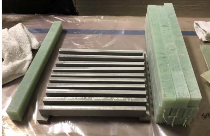
Figure 4 – Steel and composite coupons prior to assembly into DLS specimens.
