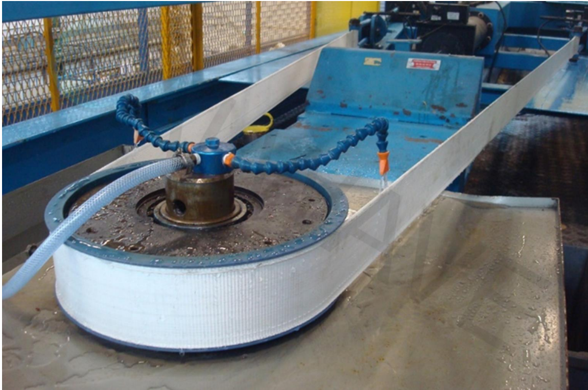
Figure 2: Experimental set up with sheave and belt mounted to the test machine.
