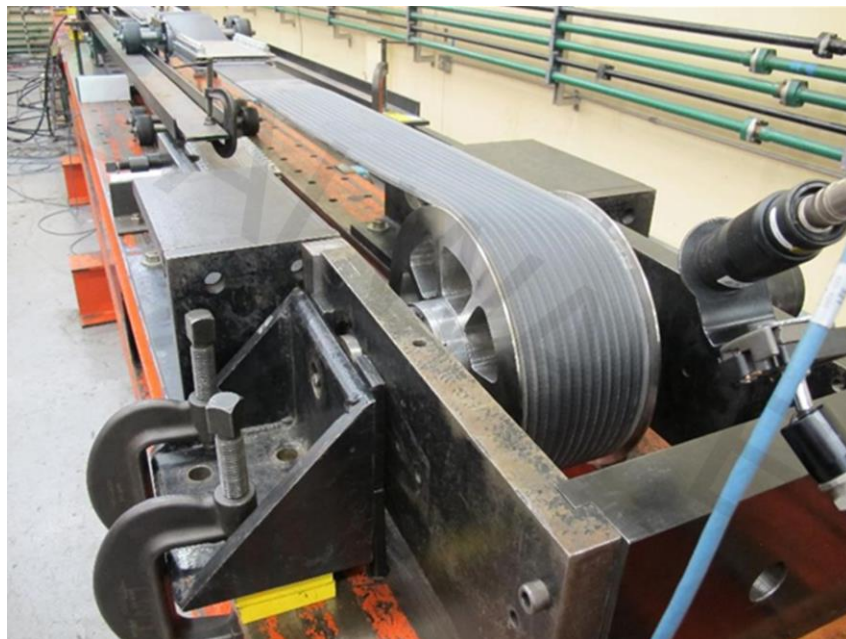
Figure 10: Drive drum and IR temperature sensor
