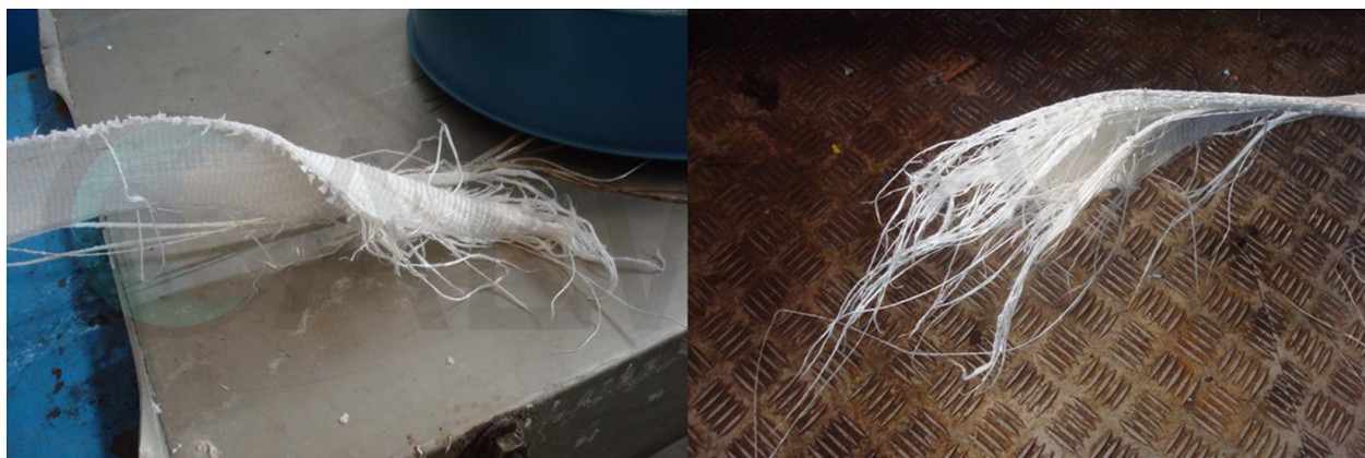
Figure 4: Belt after complete failure.
