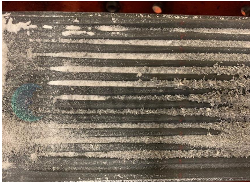
Figure 15: Belt wear residue at 847,612 machine cycles.
