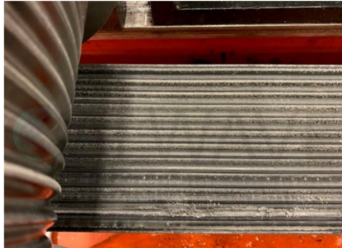
Figure 12: Drive belt wear in double bend zone after 750,962 cycles. Greatest wear on the near edge of the belt.
