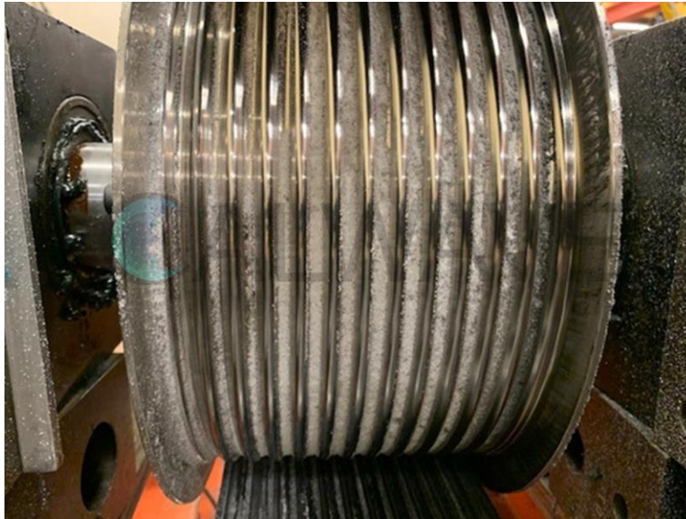
Figure 16: Belt wear debris in drum grooves at 847,612 machine cycles.
