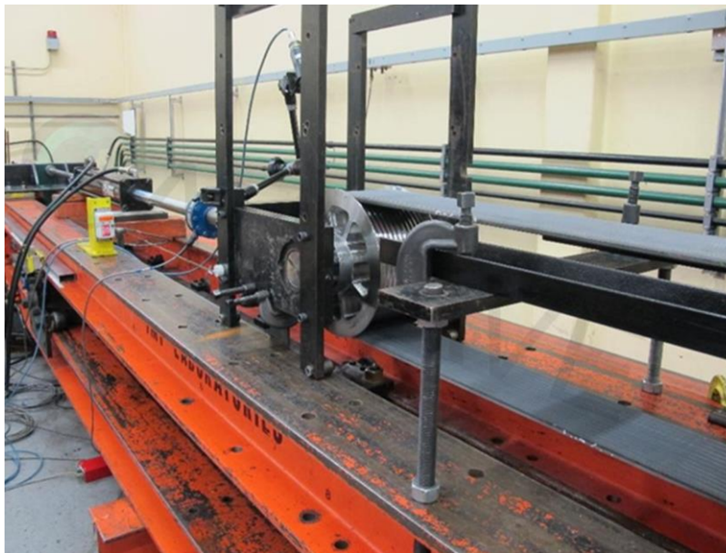
Figure 8: Tensioning drum clevis assembly attached to load cell and hydraulic tensioning cylinder.
