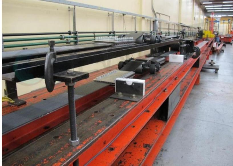
Figure 9: Belt samples attached to termination support trolleys.
