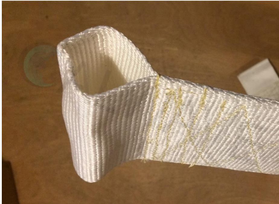
Figure 1: HMPE belt construction showing end loop termination.
