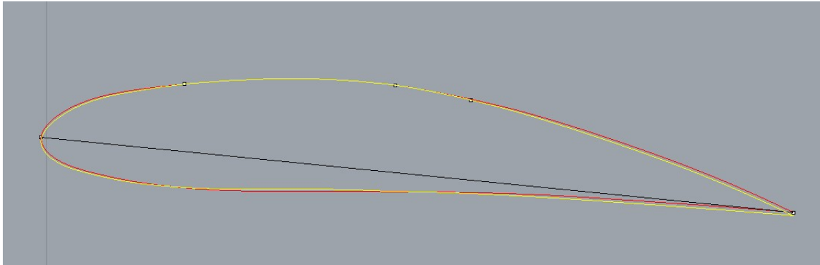
Figure 9. The original and the morphed foil profiles for the shroud of the current turbine (red: the original profile of the baseline design; yellow: the morphed profile as a design variate).
