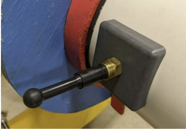
Figure 4.7: Underwater connector and patch piece subassembly fully assembled onto spar buoy.
