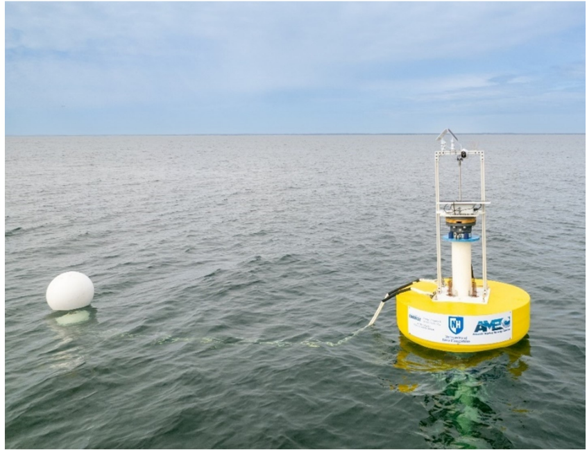
Figure 6.17: Wave pump mooring (#5), removal of winter mooring stick and rope (left), wave pump device fully deployed on mooring, facing towards NH coast (right).
