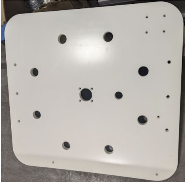
Figure 4.10: Top plate of spar buoy with updated design for DAQ module and lidar mounts and enlarged overhangs to prevent water ingress.
