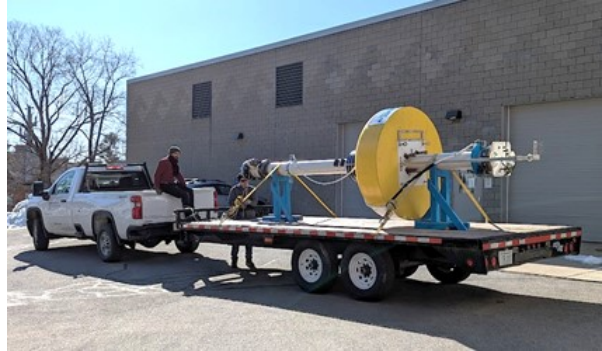
Figure 6.6: Wave pump loaded onto flatbed trailer with stands and straps.
