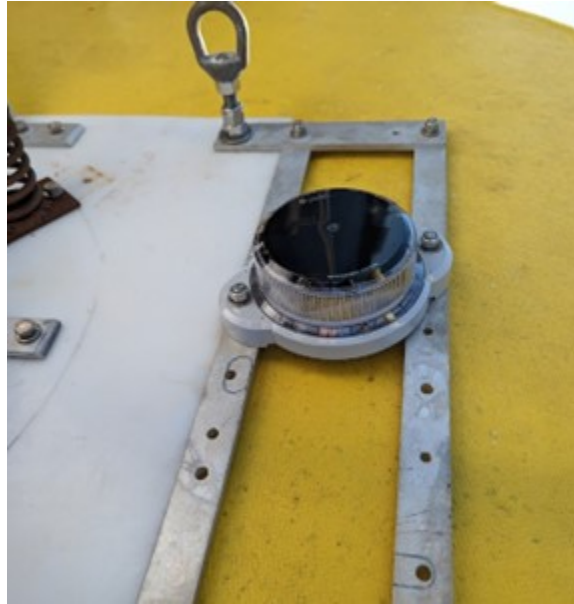
Figure 6.9: Marine Carmanah light installed onto surface float bracket for visibility at night and to meet NEPA permitting requirements.
