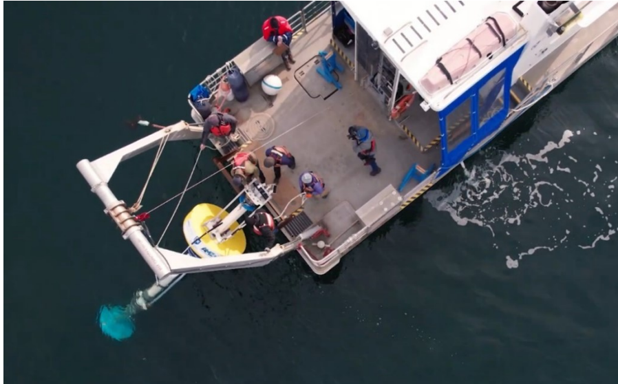
Figure 6.15: Deploying wave pump device off stern of R/V Gulf Challenger using hydraulic winch, A-frame, and quick release.
