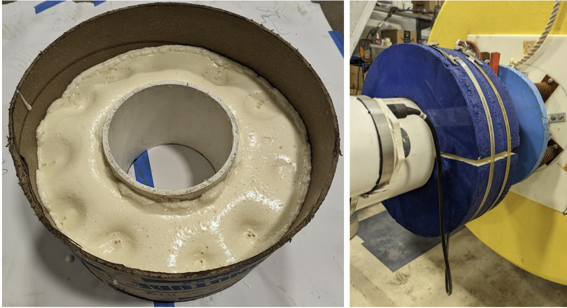
Figure 4.15: Buoyancy collar developed to achieve ideal spar equilibrium location. Manufacturing process (left), and finished result installed on spar (right).
