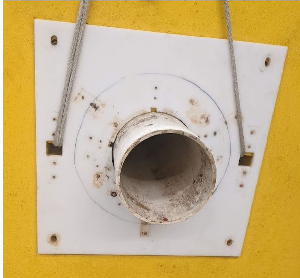
Figure 4.1: Wave pump float subassembly with corroded hardware removed.
