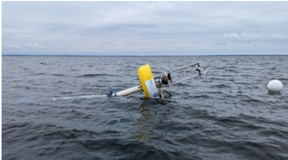
Figure 6.20: Wave pump device on mooring, stable on its side after rough wave conditions.
