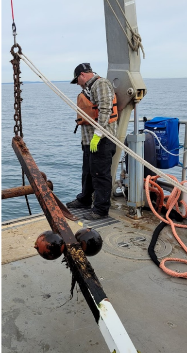
Figure 6.17: Wave pump mooring (#5), removal of winter mooring stick and rope (left), wave pump device fully deployed on mooring, facing towards NH coast (right).
