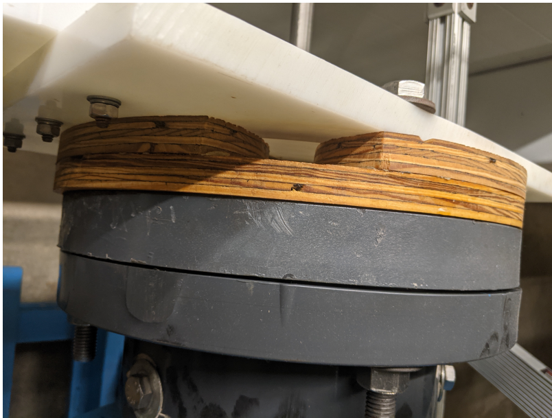
Figure 9.8: Plywood air vent component at the top of the spar buoy.
