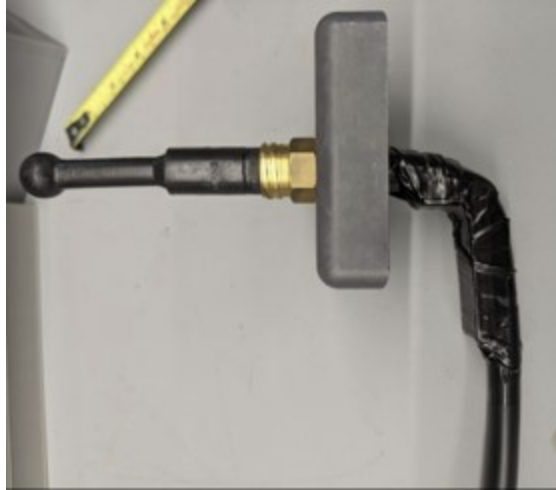
Figure 4.4: Underwater electrical connector mounted to patch part, prior to adhesion to spar buoy.
