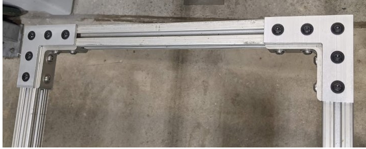
Figure 4.3: Aluminum gantry at the top of the float buoy subassembly with new aluminum brackets retrofitted.
