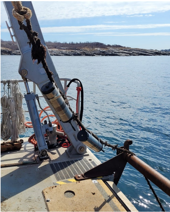
Figure 6.18: #6 mooring with hydrophones installed onto rope (left), Sofar Spotter buoy and mooring fully installed (right).
