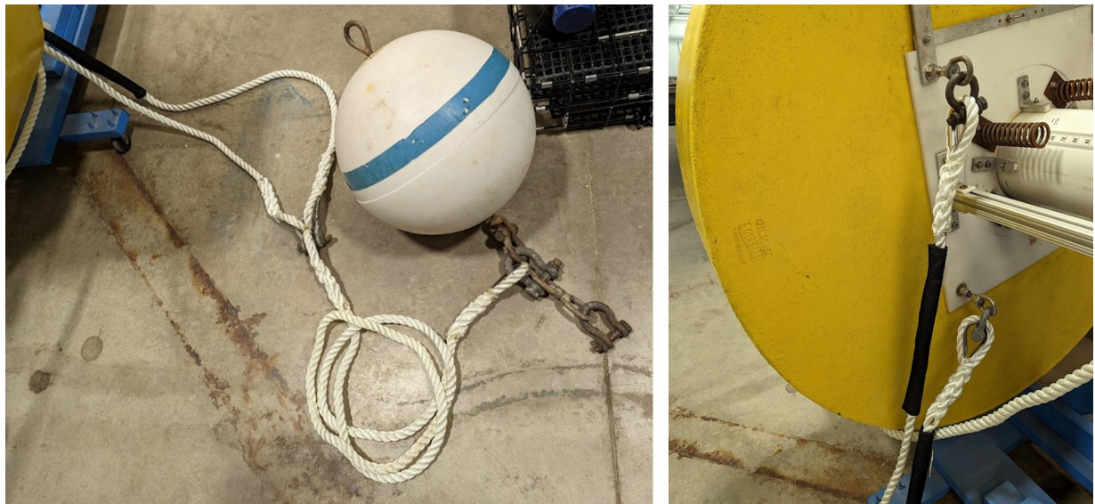
Figure 6.4: Wave pump mooring components prior to deployment. Y-shape bridle and long mooring line connect to swivel, shackles, and buoy (left). Y-shape bridle connections to float eyehooks with shackles (right).
