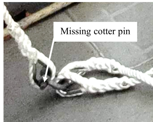
Figure 6.21: Wave pump device ashore on Appledore Island, ME, March 31st, 2023 (left). Shackle with missing cotter pin during deployment process March 21st, 2023 (right).
