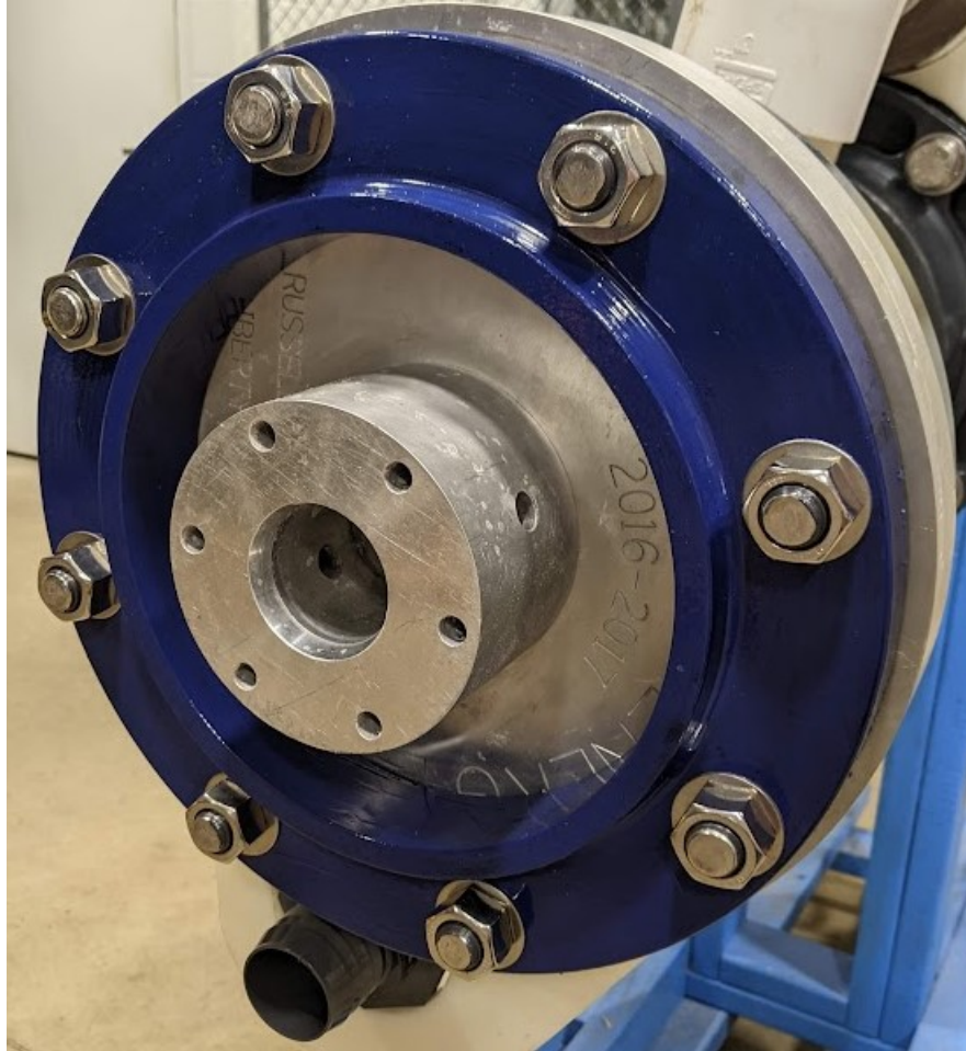
Figure 4.11: Ballast weight of twenty-six pounds incorporated directly onto spar buoy using OTS steel pipe flange, coated in marine-grade anti-corrosion paint.
