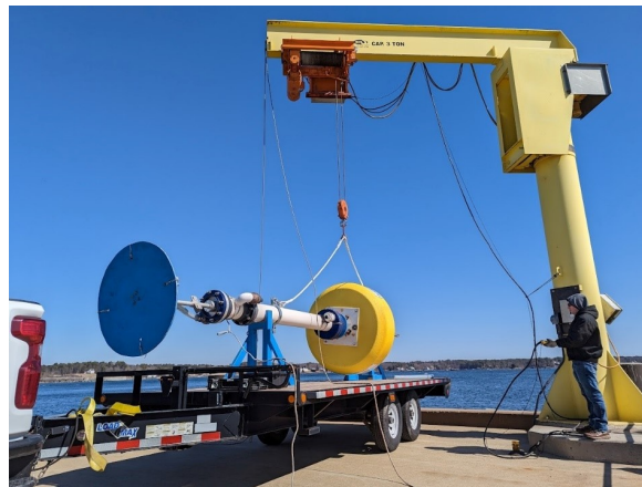
Figure 6.7: Unloading the wave pump device from the trailer using the crane pier.
