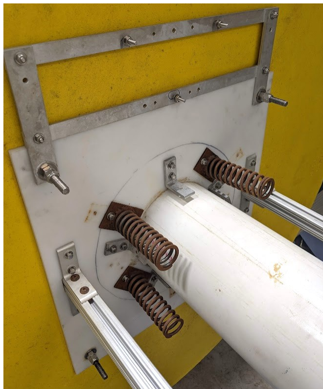
Figure 4.2: Wave pump float subassembly with new 316 Stainless Steel hardware installed.
