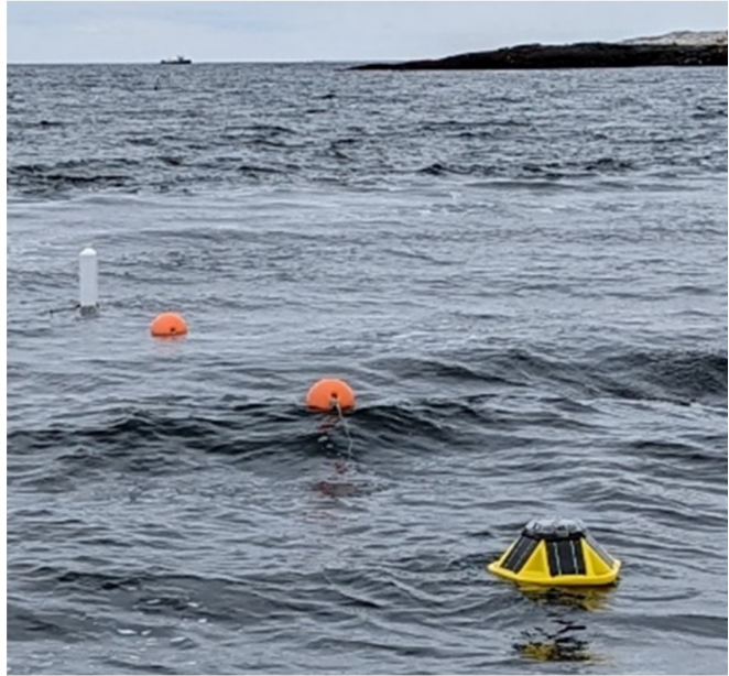
Figure 6.18: #6 mooring with hydrophones installed onto rope (left), Sofar Spotter buoy and mooring fully installed (right).
