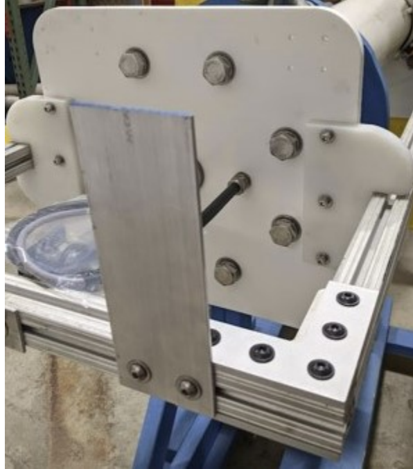
Figure 4.12: Aluminum lidar target mounted onto float buoy's aluminum gantry.
