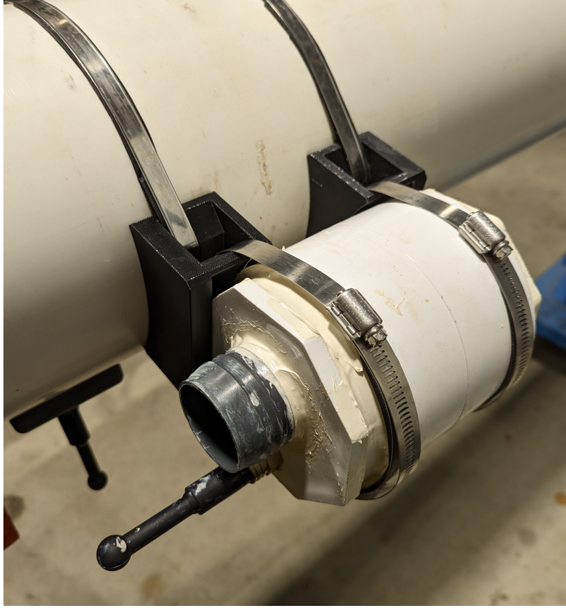
Figure 4.9: Flow meter housing installed onto spar buoy.
