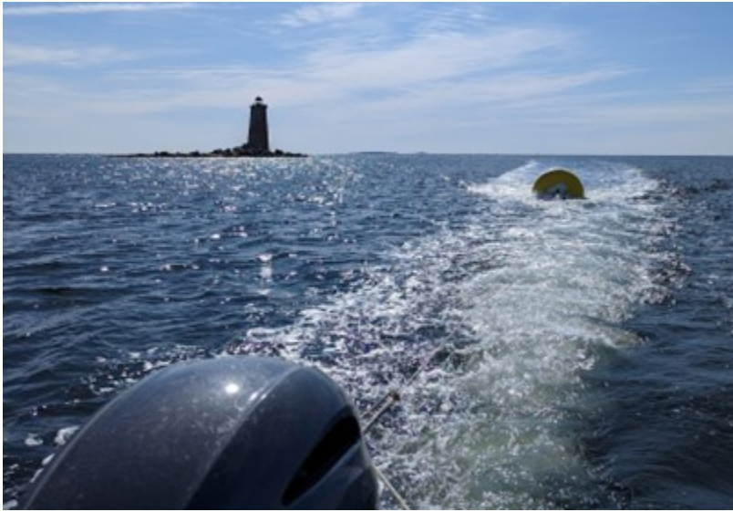
Figure 6.22: Towing wave pump device to New Castle, NH using Galen J vessel.
