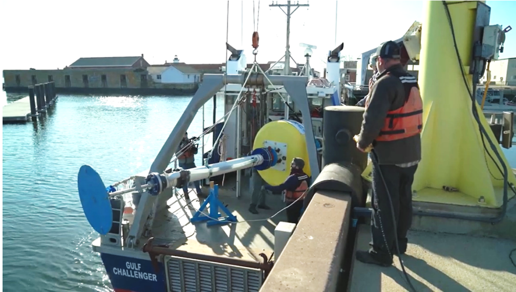
Figure 6.13: Loading wave pump device onto R/V Gulf Challenger using pier crane, facing towards ship. Vertical riser stands (two used, one shown) on ship deck to support device.
