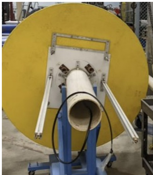
Figure 4.6: Underwater electrical connector cable routed to top of the spar buoy. Shown in picture by black cable.
