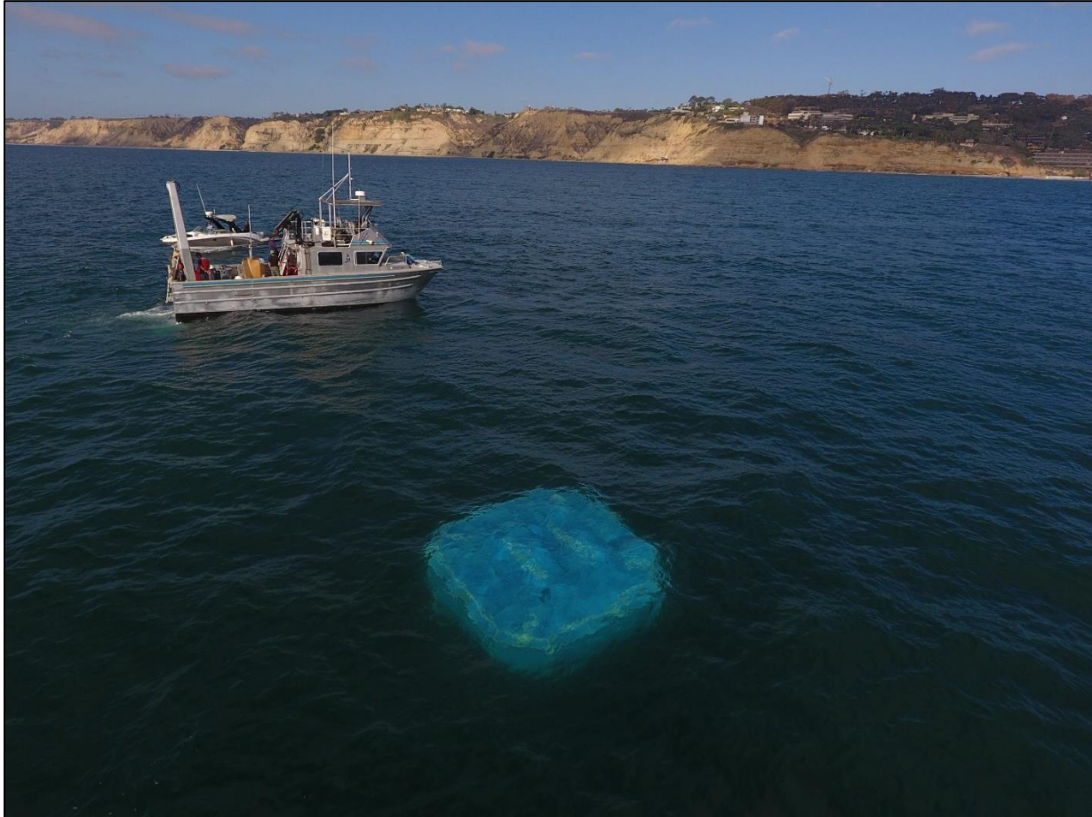
Figure 1: CalWave's xWave Technology deployed at Scripps, CA, operating fully submerged.
