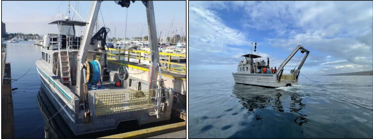
Figure 25: Left: RV Beyster with loaded umbilical reel. Right: RV Beyster during spool out of the umbilical.
