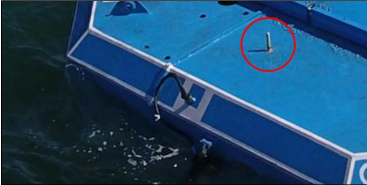
Figure 35: Wi-Fi antenna installed on deployed x1.
