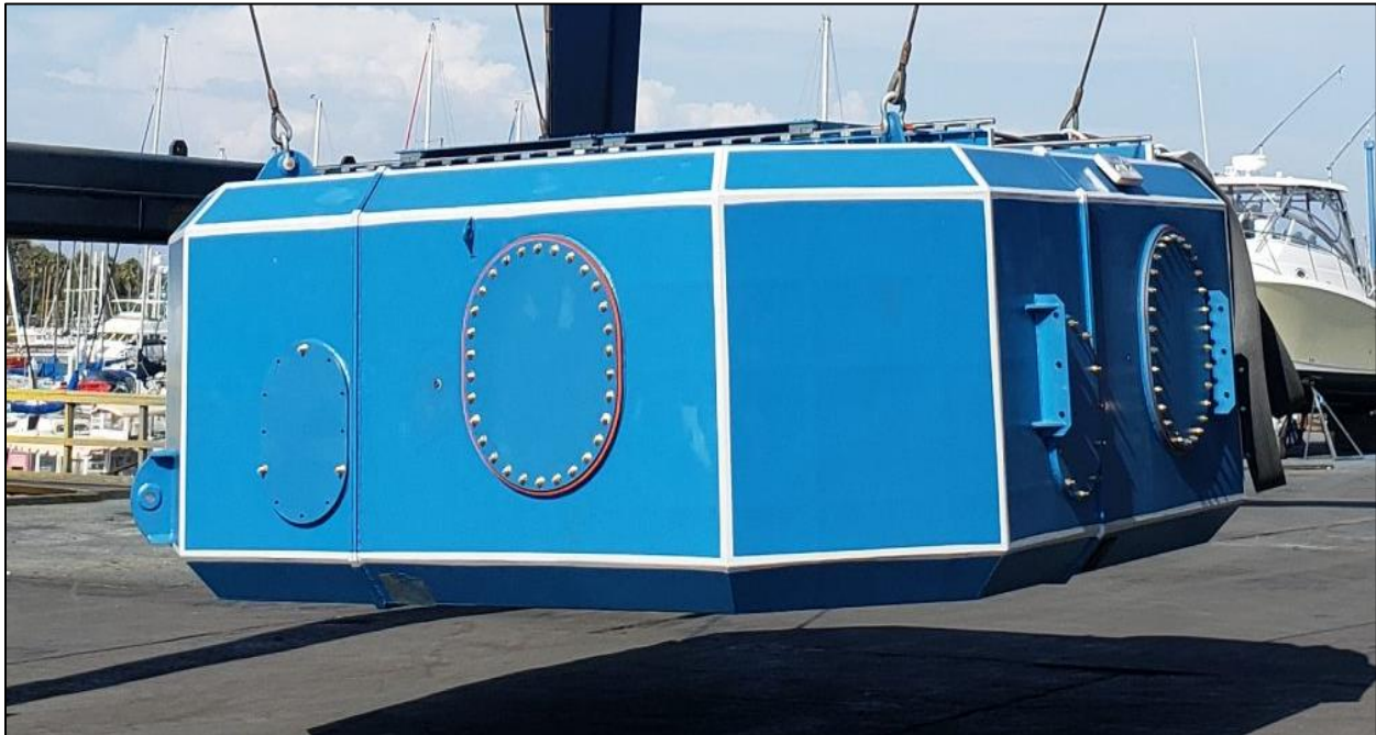
Figure 12: X1’s prismatic absorber body during a lifting operation.
