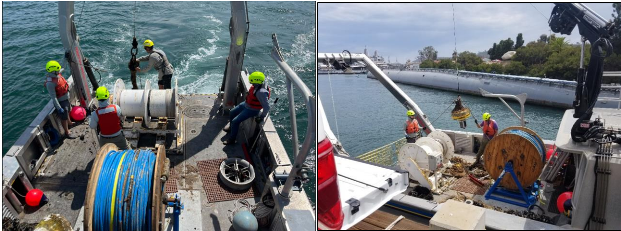
Figure 27: Recovery operation of the umbilical on the RV Beyster with CalWave staff.
