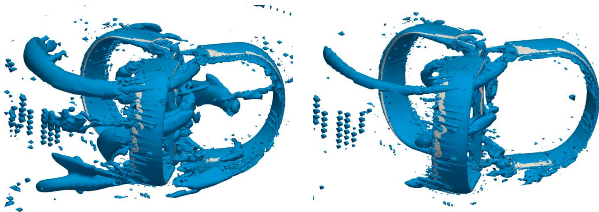
(b) Rotor at wave trough (left: Q-criterion = 3; right: Q-criterion = 10)
