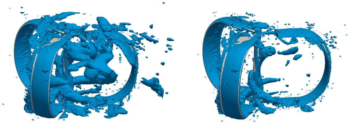
(a) Rotor at wave crest (left: Q-criterion = 3; right: Q-criterion = 10)
