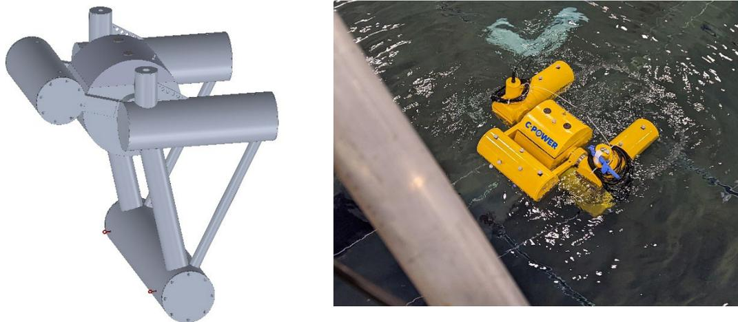
Figure 71 – Schematic depicting H3 scaled model (left), and photo of deployed model (right).
