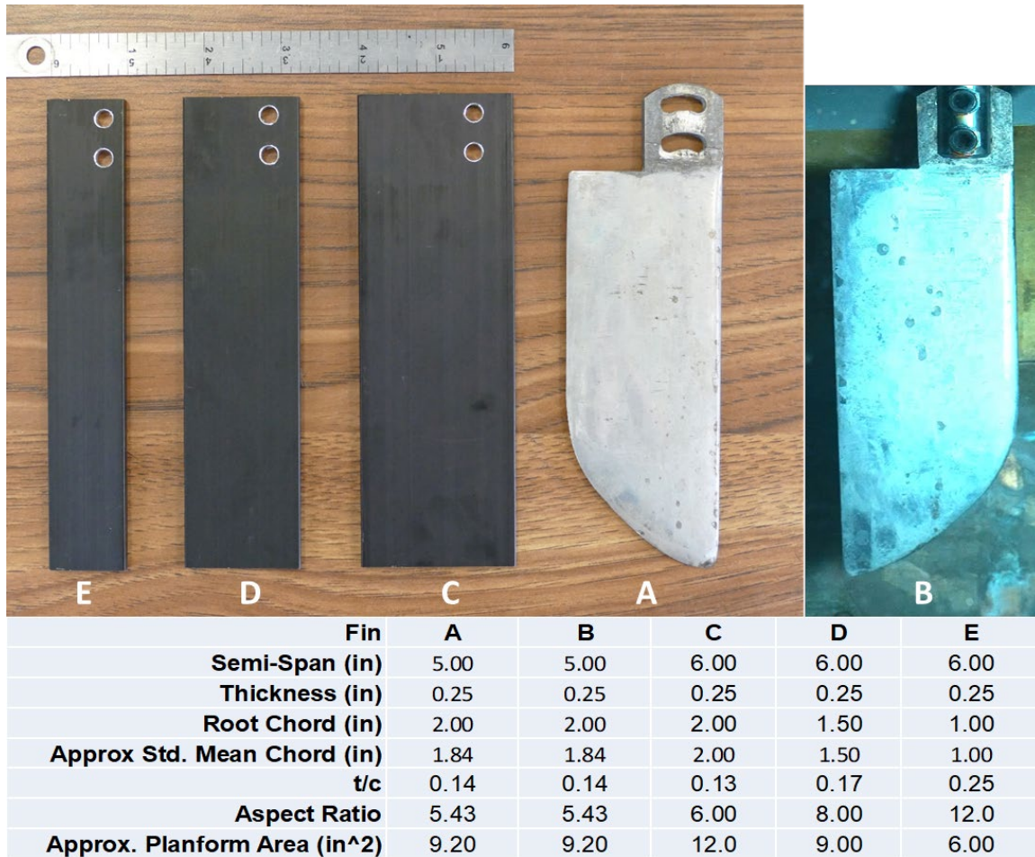
Figure 8: Hydrofoil/fins provided by Pterofin with geometric parameters
