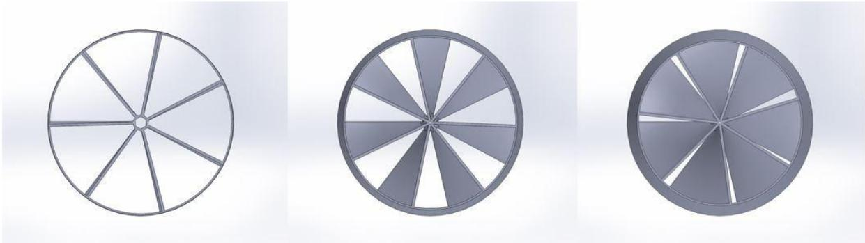
**Figure 2.** Sitkana's integrated shrouded turbine geometry, illustrating that it can be formed by repetitively stacking the initial shape, twisting and shrinking each layer.
