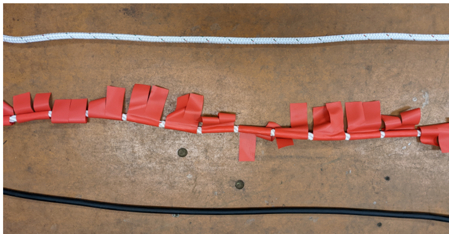
2170 Fig. B4 (top) Low-stretch nylon cord, (middle) low-stretch nylon cord with vinyl tape fairing (3M 2171 3903), (bottom) standard rubber cord. All cords are 9.53 mm (3/8 in) in diameter.
