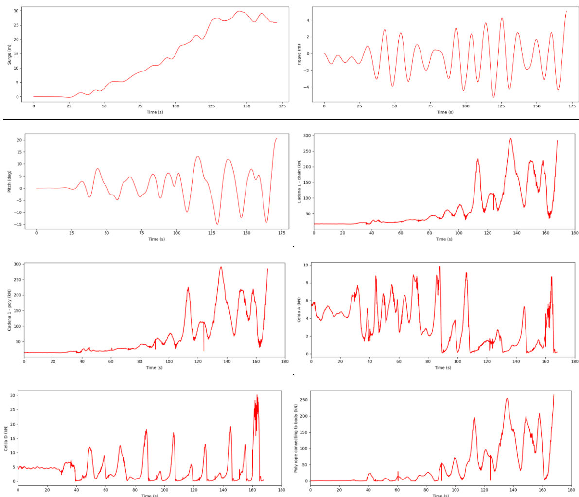
Figure 23: H601 Fully Coupled Simulation of Full Size Model with Different Mooring System- Illustrations of the body motion along with the mooring tensions when the WEC is subjected to a period of 170 s of high wave elevations.
