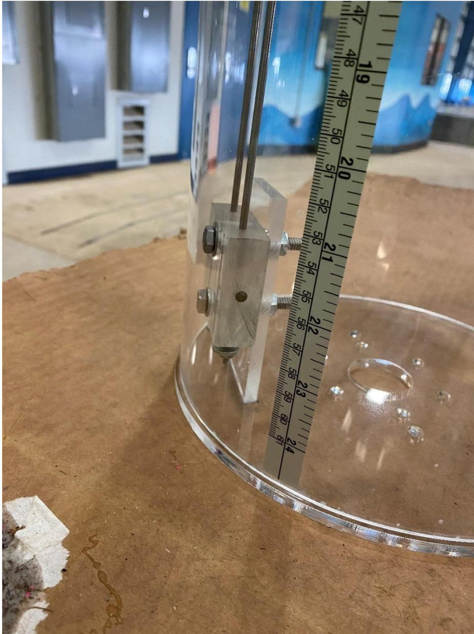
Figure D.6. Close up image of surface elevation probe with waterproof gradation tape.
