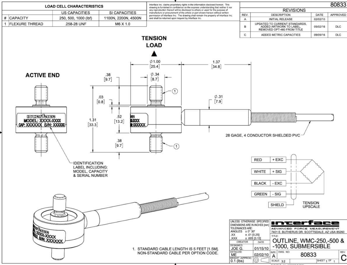
Figure A.3. WMC-500 Load Cell
