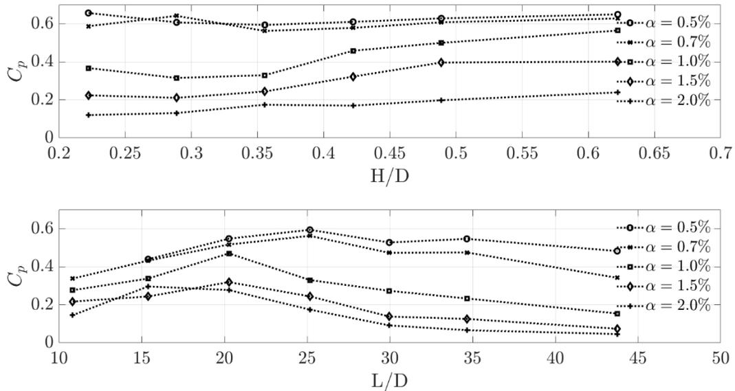
Figure 7.1.6 Normalized Fixed Model Pressure Drop. (Top) Normalized relative to a change in wave height. (Bottom) Normalized relative to change in wavelength.  $C_p$  represents the differential pressure across the orifice, normalized by the hydrostatic pressure of the wave. For changes in amplitude, a wave period of 2 seconds is assumed. For changes in wavelength, a wave height of 8 cm is assumed.
