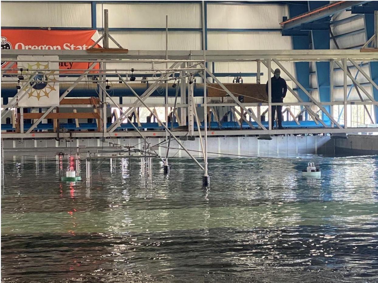
**Figure 6.1.3. Wave Basin Shore Side View. (Left) Floating Test Article. (Right) Fixed Test Article.**
