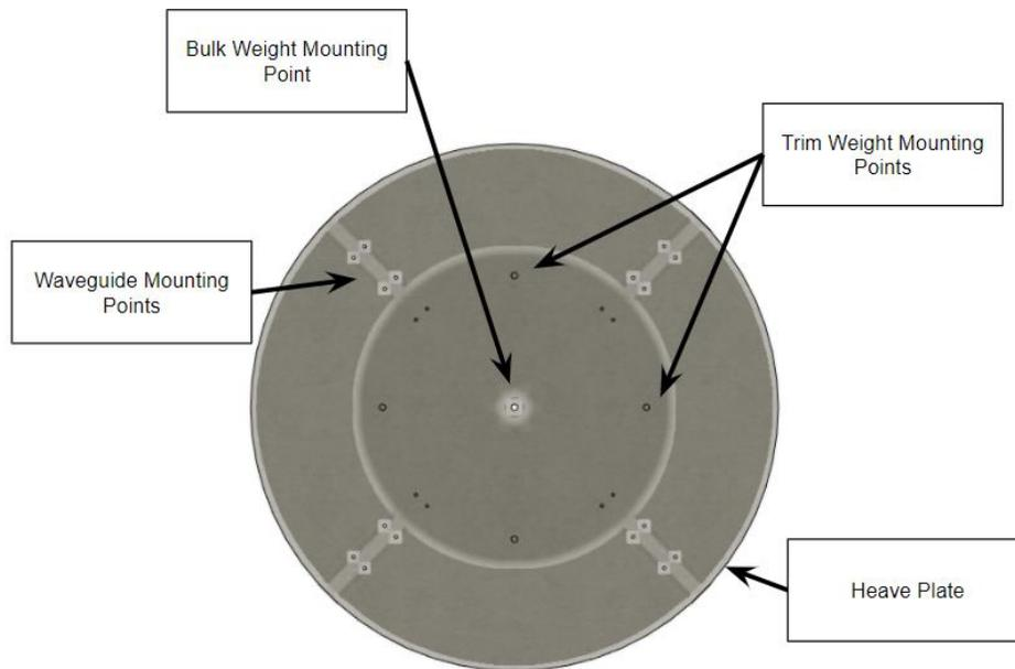
Figure 5.1.3 Floating Test Article Heave Plate Mounting Points
