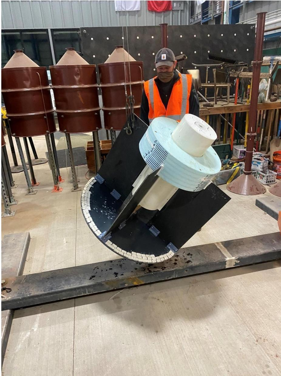
Figure D.2 Center of Gravity Hang Testing.
