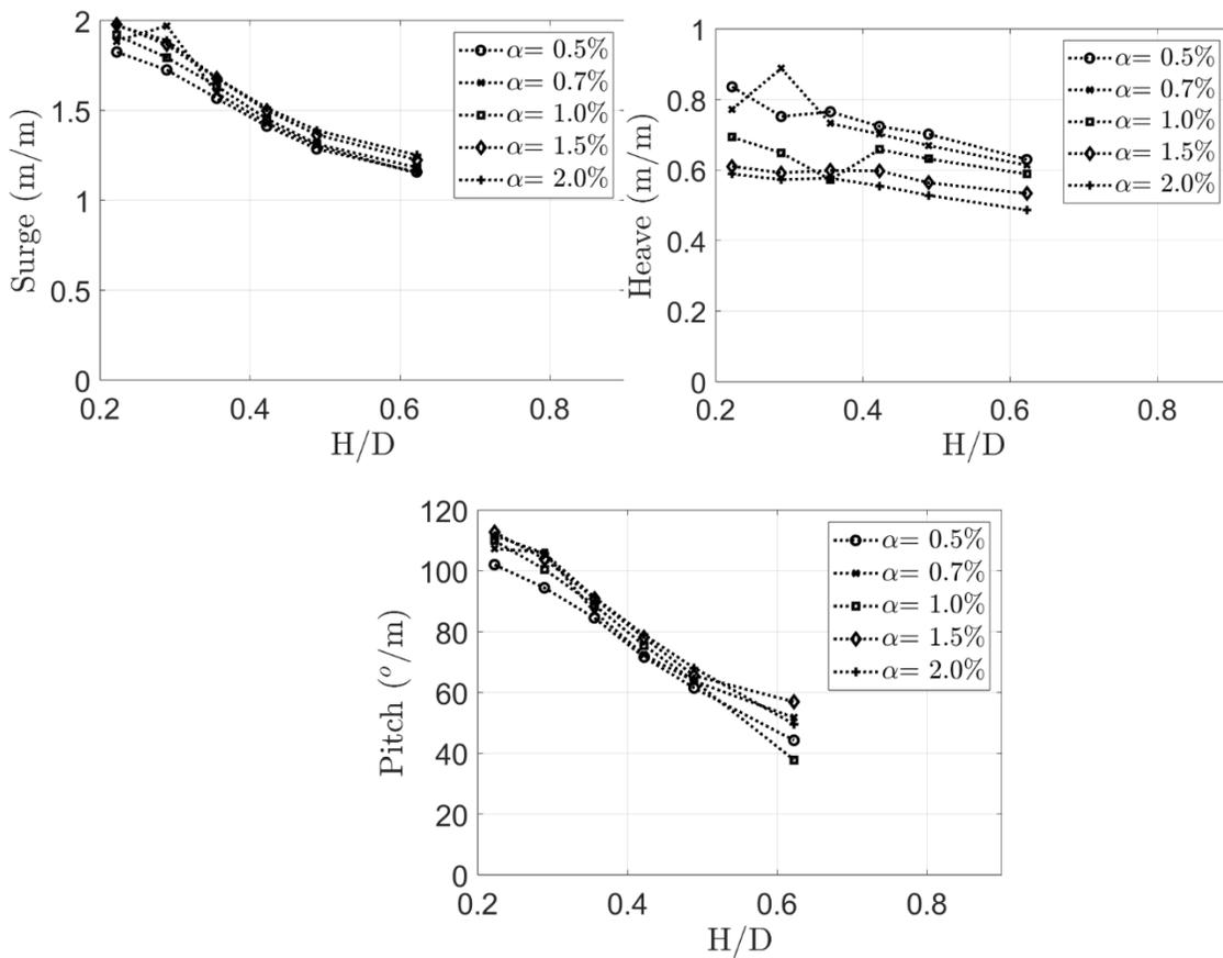
Figure 7.1.2 Amplitude dependent motion response for (Top Left) Surge, (Top Right) Heave, and (Bottom) Pitch. D represents the diameter of the OWC chamber, while L is the wavelength.
