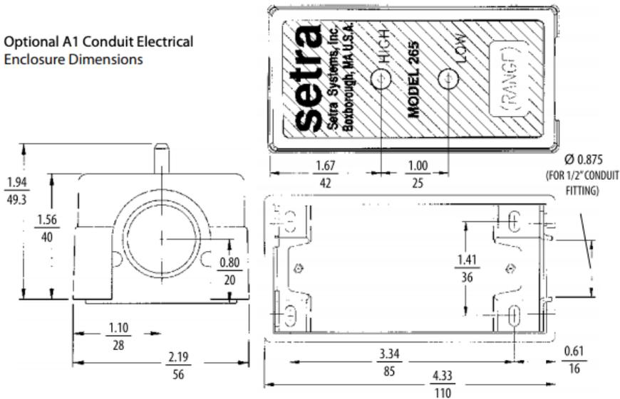
Figure A.2. Setra Very Low Differential Pressure Sensor Dimensions.
