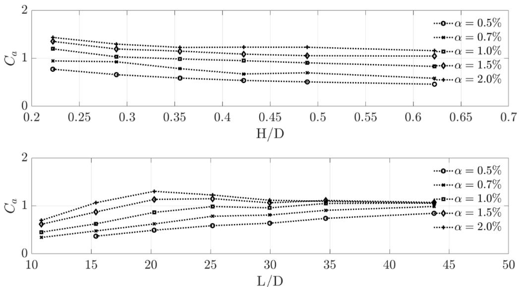
Figure 7.1.7 Normalized Fixed Model Surface Amplification. (Top) Normalized relative to a change in wave height. (Bottom) Normalized relative to change in wavelength.  $C_a$  represents the internal surface displacement range, normalized by the regular wave height. For changes in amplitude, a wave period of 2 seconds is assumed. For changes in wavelength, a wave height of 8 cm is assumed.
