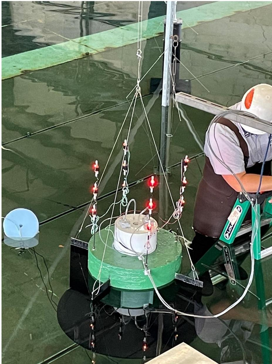
Figure D.4. Heave Decay Test Set up.
