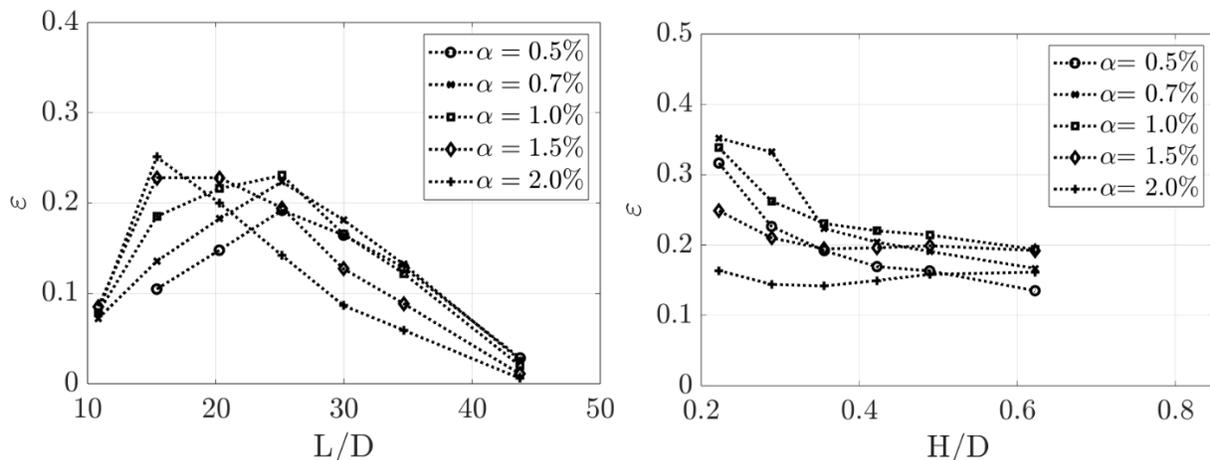
Figure 7.1.3 Normalized Floating Model Efficiency. (Left) Normalized relative to a change in wave height. (Right) Normalized relative to change in wavelength. Lines represent the percentage opening ratio.
