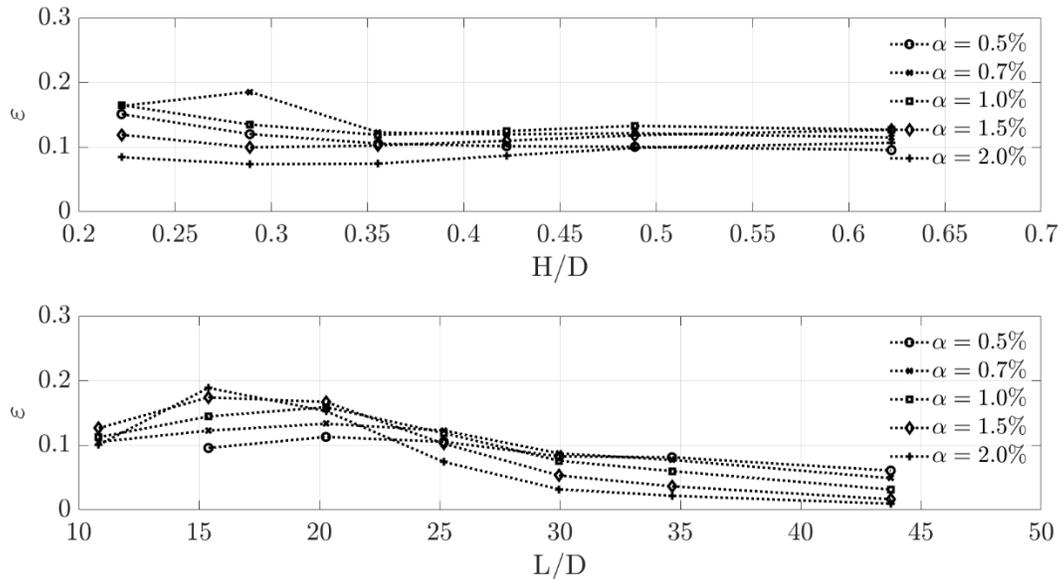
Figure 7.1.4 Normalized Fixed Model Capture Efficiency. (Top) Normalized relative to a change in wave height. (Bottom) Normalized relative to change in wavelength.
