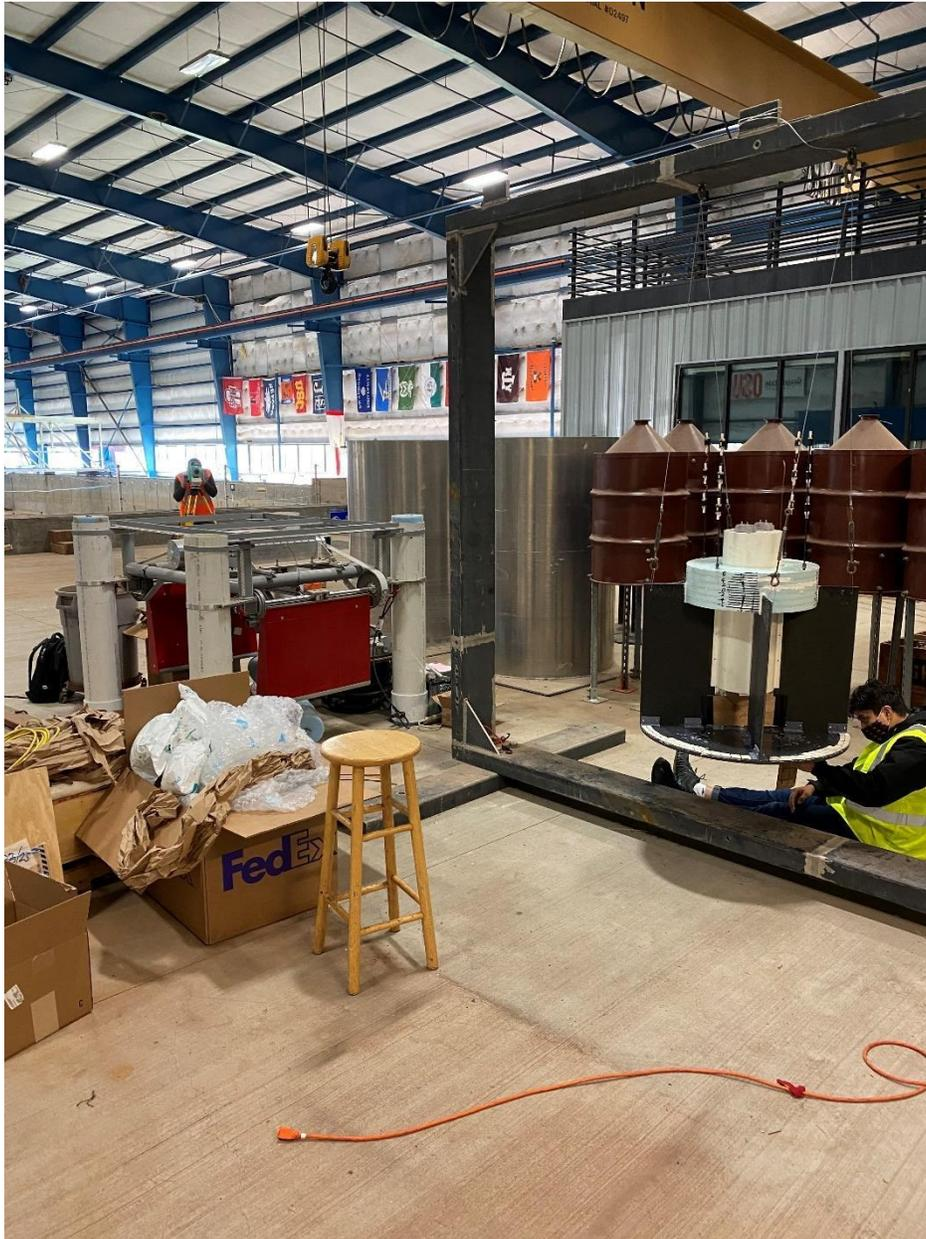
Figure D.3 Model Coordinate Surveying. Test Set up used in Compound Pendulum test to determine the radius of gyration.
