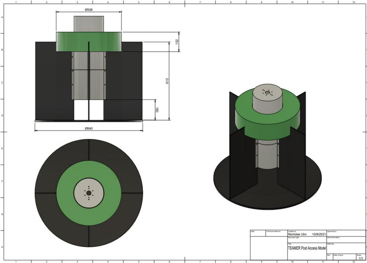
Figure 5.1.2 Drawing of Floating Test Article. Dimensions in mm
