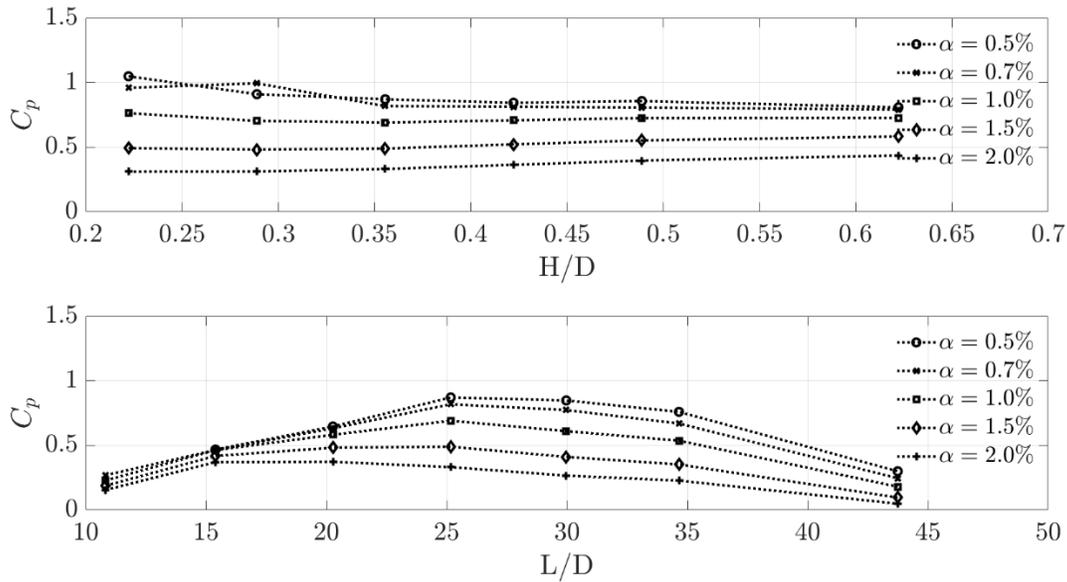
Figure 7.1.5 Normalized Floating Model Pressure Drop. (Top) Normalized relative to a change in wave height. (Bottom) Normalized relative to change in wavelength.  $C_p$  represents the differential pressure across the orifice, normalized by the hydrostatic pressure of the wave. For changes in amplitude, a wave period of 2 seconds is assumed. For changes in wavelength, a wave height of 8 cm is assumed.
