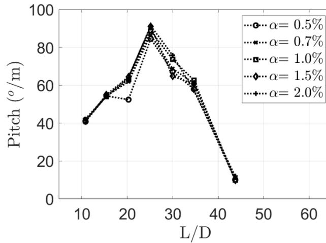
Figure 7.1.1 Response Amplitude Operators for (Top Left) Surge, (Top Right) Heave, and (Bottom) Pitch. D represents the diameter of the OWC chamber, while L is the wavelength.
