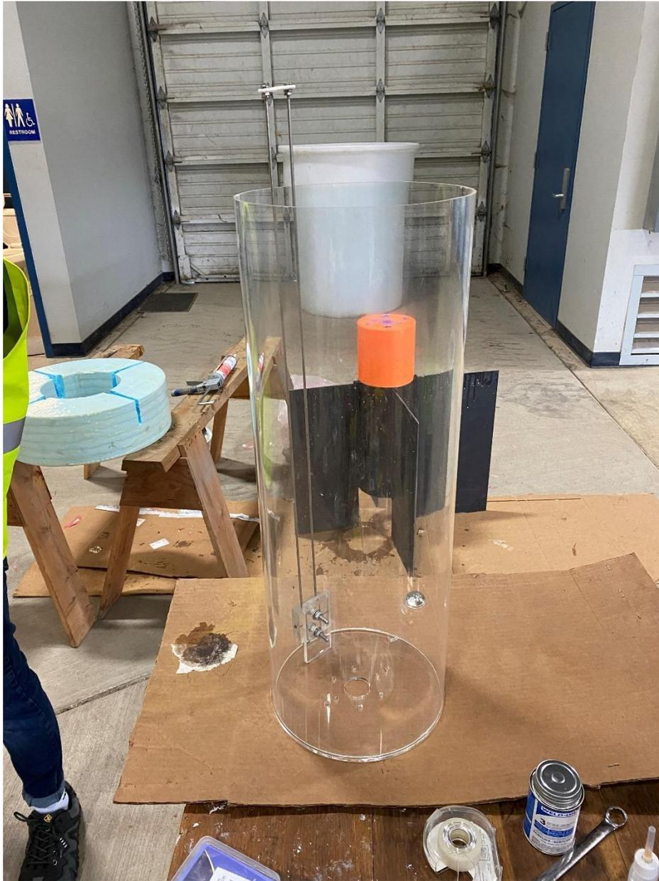
Figure D.5. Fixed Model Surface Elevation Probe Installation.
