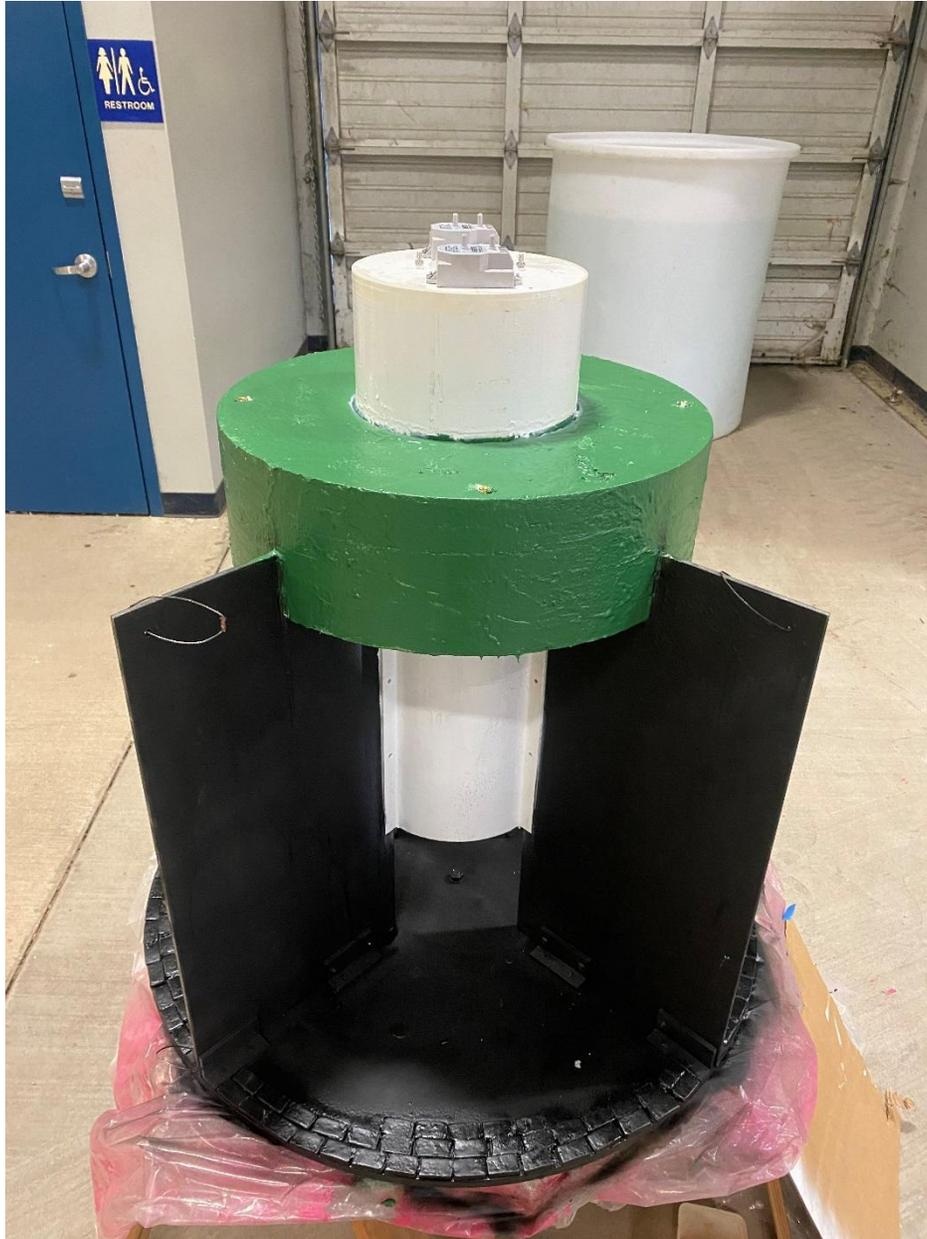
Figure 5.1.1 Image of Floating Test Article at O.H. Hinsdale Wave Research Lab. Bricks along the heave plate edge are trim weights. Differential Pressure Sensors affixed to the top of the model.
