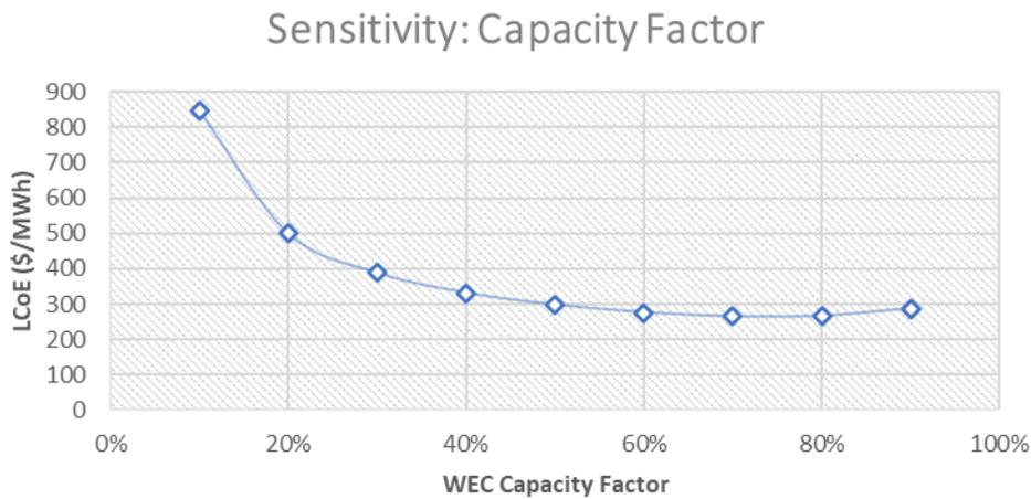
Figure 36 - LCoE Sensitivity to Capacity Factor
