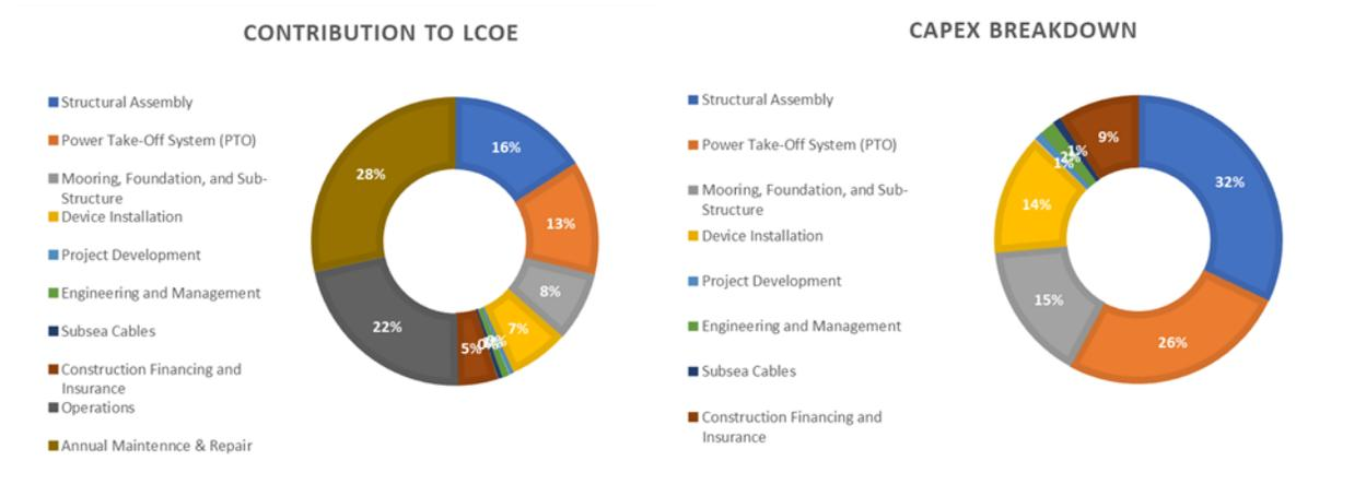
Figure 47 - 100MW Capex and LCoE by Cost Center for Waveswing
