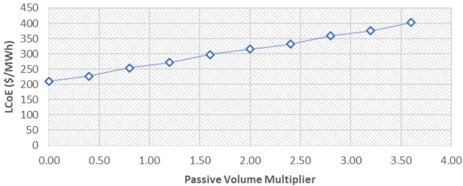
Figure 17 - Passive Volume Multiplier vs. LCoE.
