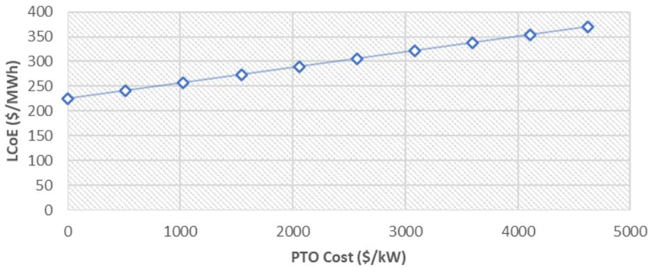
Figure 25 - LCoE Sensitivity to PTO Capex
