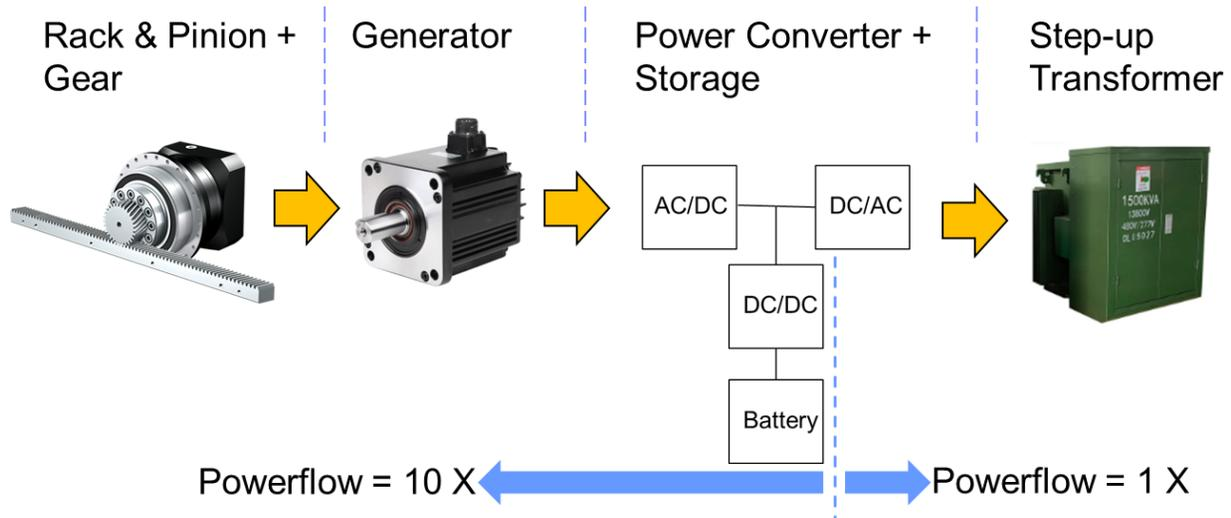
Figure 11 -Direct-Drive PTO Topology
