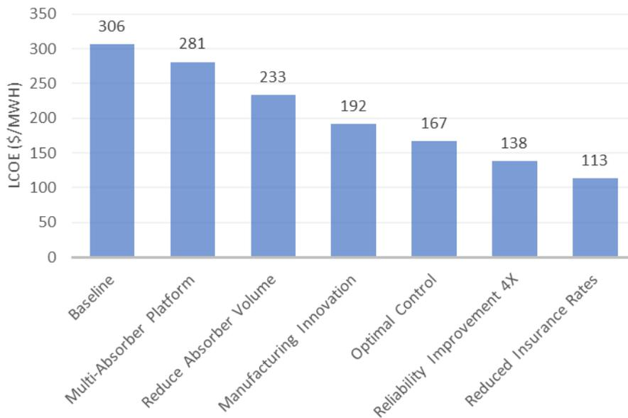
Figure 30 - Cost Reduction Pathway for AWS Waveswing
