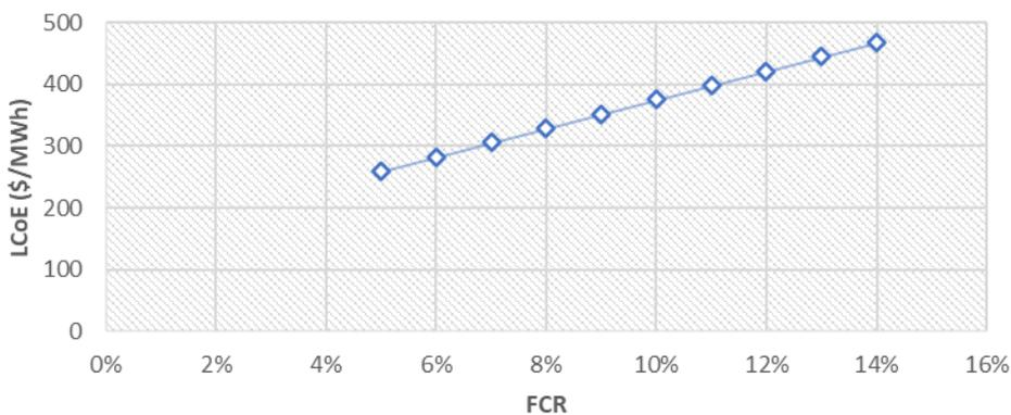
Figure 29 - LCoE Sensitivity to Fixed Charge Rate
