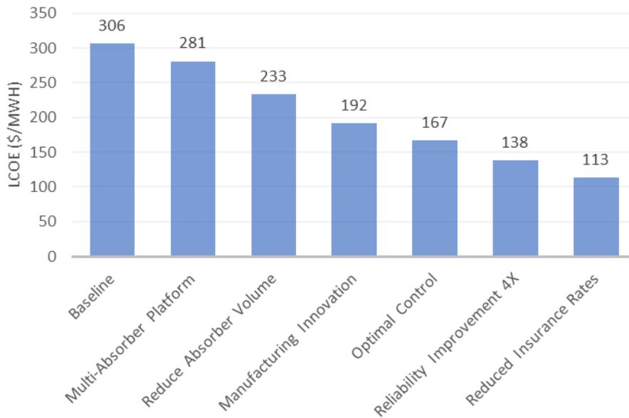
Figure 3 - LCoE Cost Reduction Pathway for Waveswing WEC
