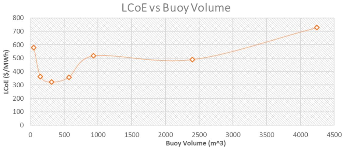
Figure 34 – LCoE vs. device active volume
