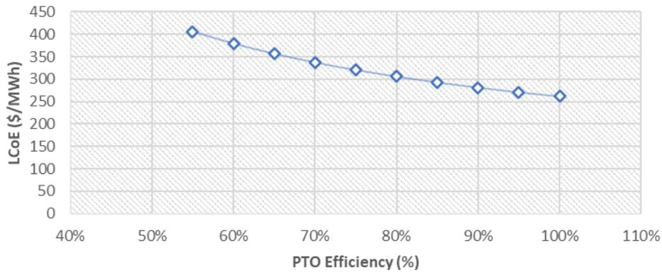
Figure 21 – LCoE Sensitivity to PTO Efficiency
