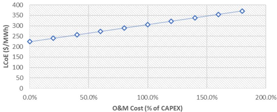
Figure 27 - LCoE Sensitivity to O&M Cost
