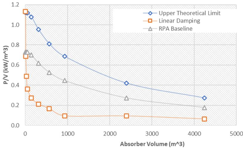
Figure 33 - Power production comparison
