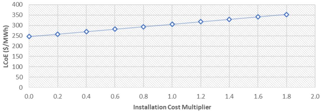
Figure 26 - LCoE Sensitivity to Installation Cost
