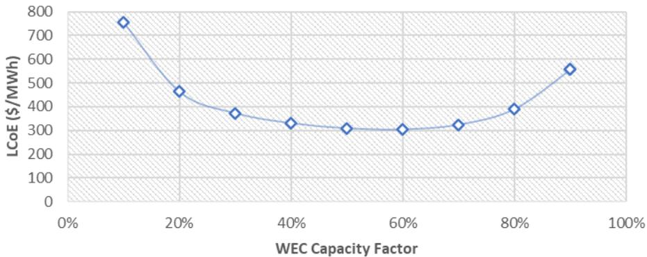
Figure 20 - LCoE Sensitivity to Capacity Factor
