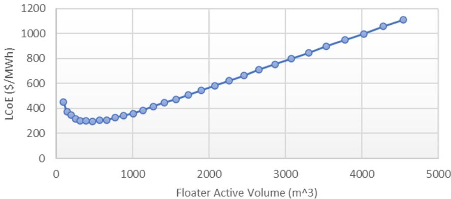
Figure 15 – LCoE vs. device active volume
