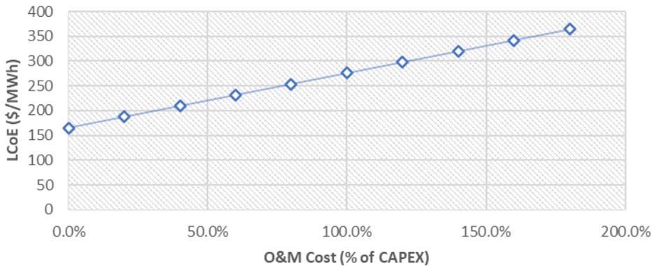
Figure 42 - LCoE Sensitivity to O&M Cost
