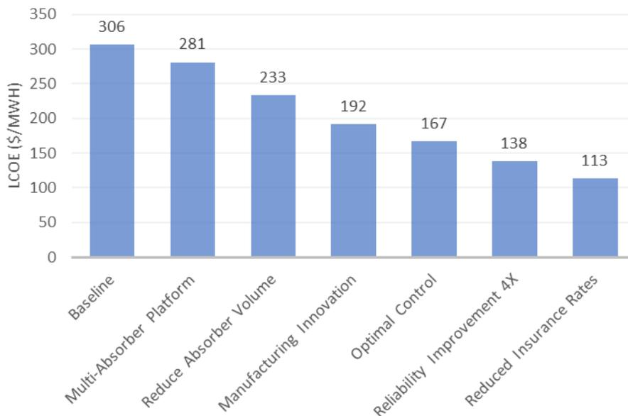
Figure 49 - LCoE Cost Reduction Pathway for Waveswing WEC
