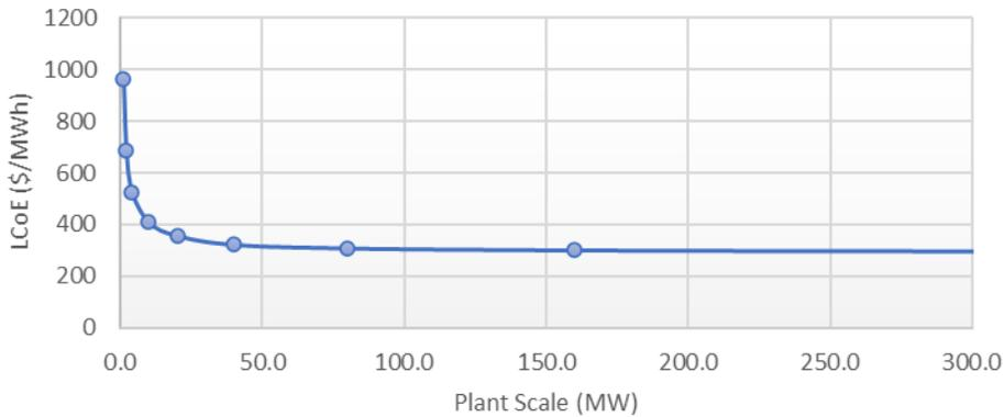
Figure 19 - LCoE Sensitivity to Plant Scale
