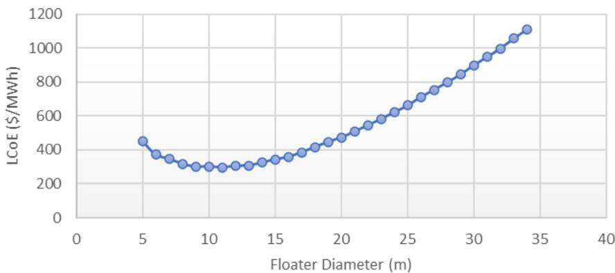
Figure 16 - Floater diameter vs. LCoE using a fixed stroke of 5m.
