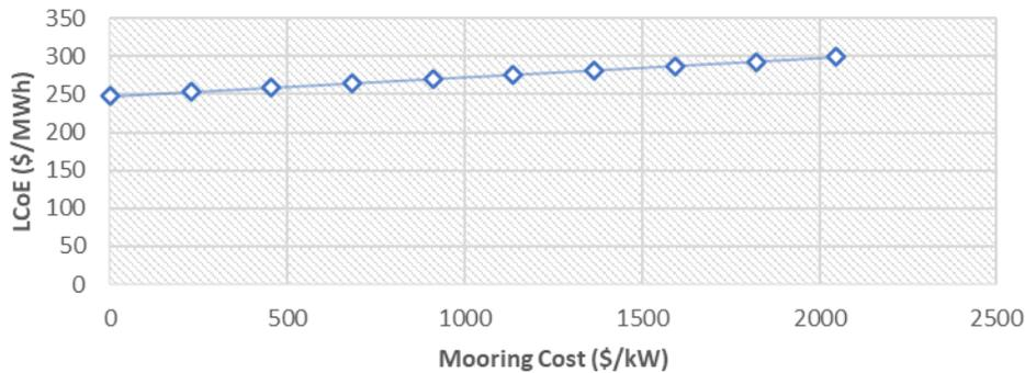
**O&M, Installation, and Insurance Cost** - Other key cost drivers affecting the LCoE include the installation, O&M, and insurance rates. The installation cost baseline was explicitly computed for this device and includes assumptions on equipment day rates and installation process timelines. Given the early-stage nature of the current design, O&M and insurance costs were estimated parametrically.
