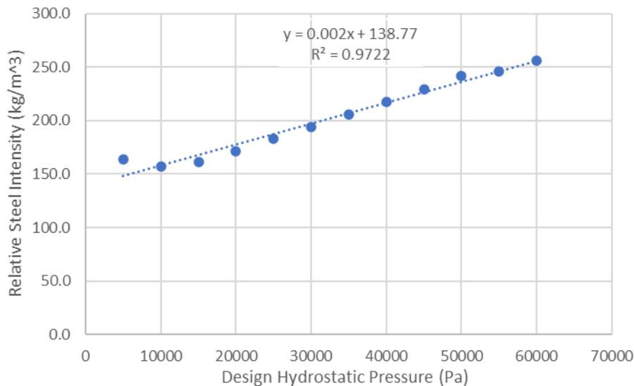
Figure 7 – Normalized steel weight as a function of barge height
