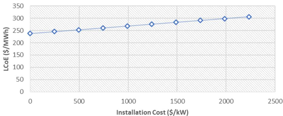
Figure 41 - LCoE Sensitivity to Installation Cost
