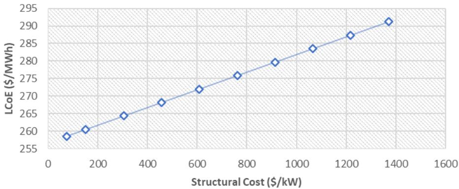
Figure 39 - LCoE vs. Structural Steel Mfg Cost
