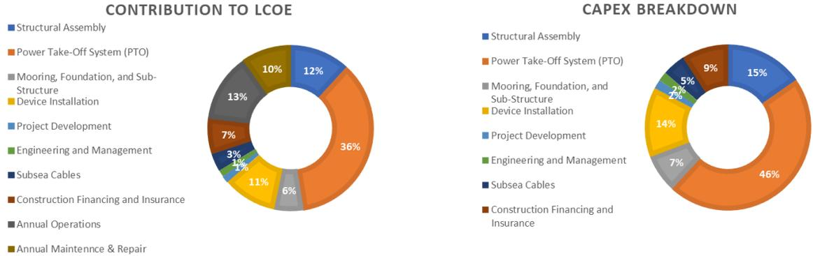
Figure 31 - LCoE and Capex Breakdown of Optimized 100MW Waveswing Plant.
