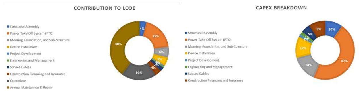
Figure 48 - 100MW Capex and LCoE by Cost Center for Reference Point Absorber
