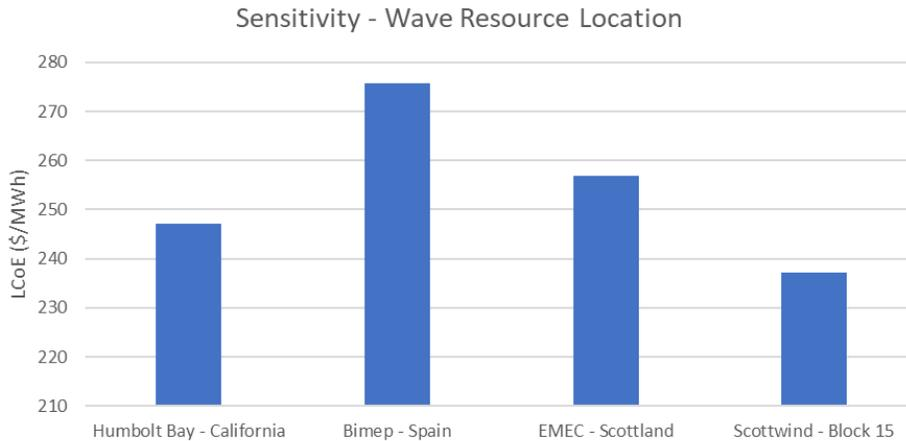
Figure 38 - LCoE Sensitivity to Wave Energy Resource
