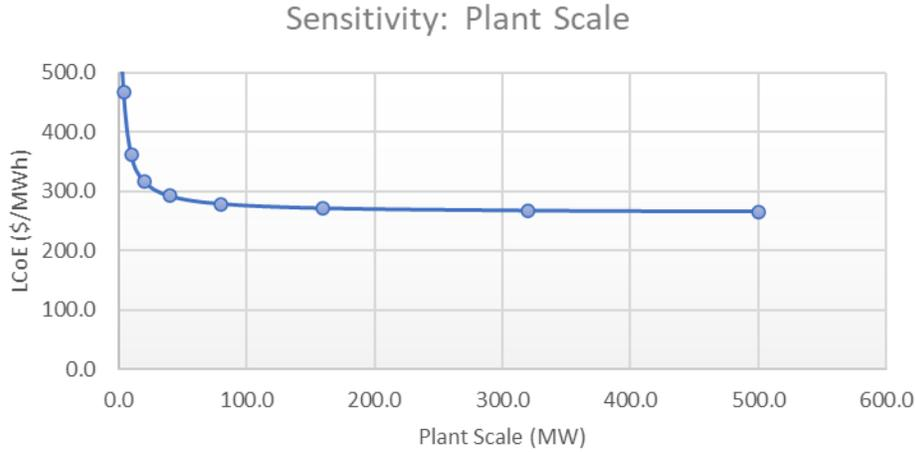
Figure 35 - LCoE Sensitivity to Plant Scale
