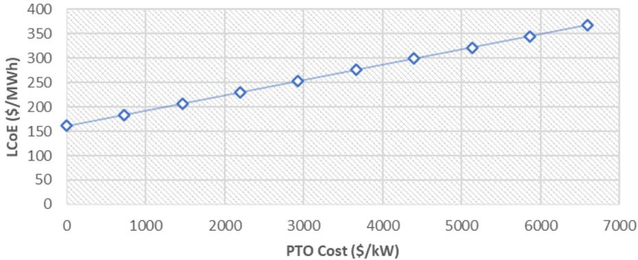
Figure 40 - LCoE Sensitivity to PTO Capex
