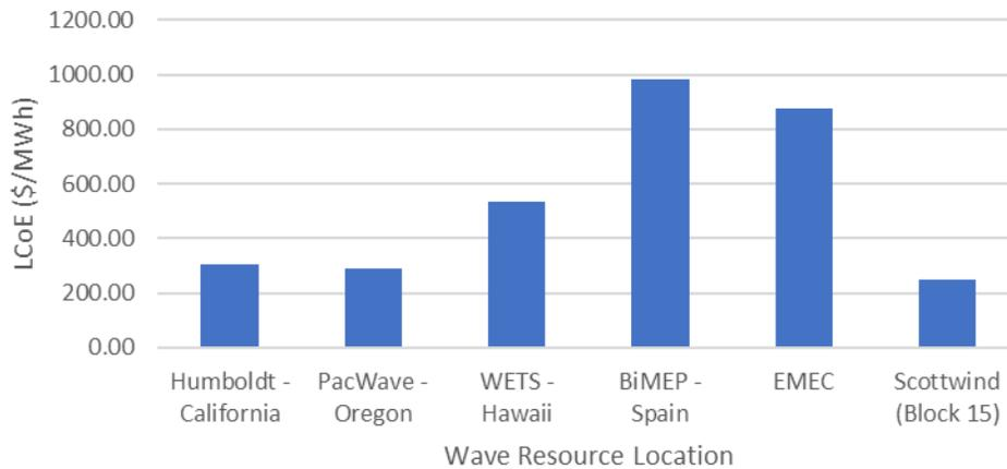
Figure 23 - LCoE Sensitivity to Wave Energy Resource
