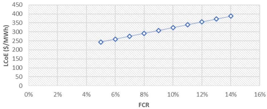
Figure 44 - LCoE Sensitivity to Fixed Charge Rate
