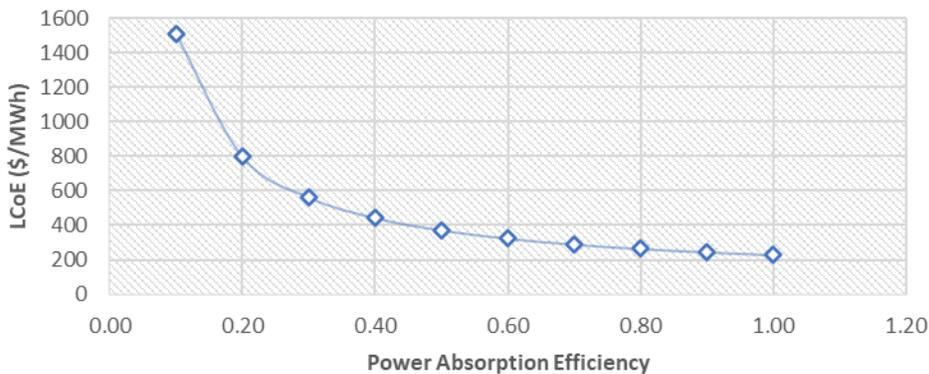
Figure 18 - LCoE vs power absorption efficiency
