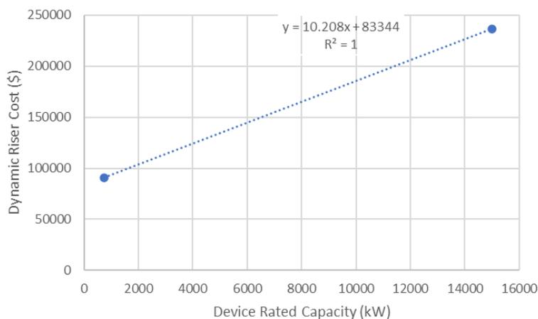
Figure 12 - Riser Cable Cost Correlation Function
