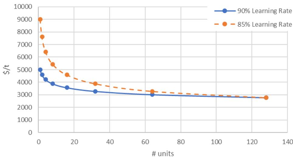
Figure 10 - Comparison of Learning Rates for Steel Manufacturing
