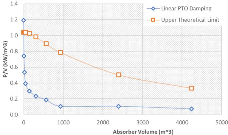
Figure 5 - P/V values for a range of different absorber volumes
