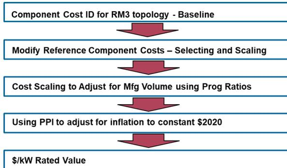
Figure 8 - Cost Estimation Process
