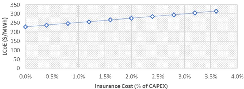
Figure 43 - LCoE Sensitivity to Insurance Cost
