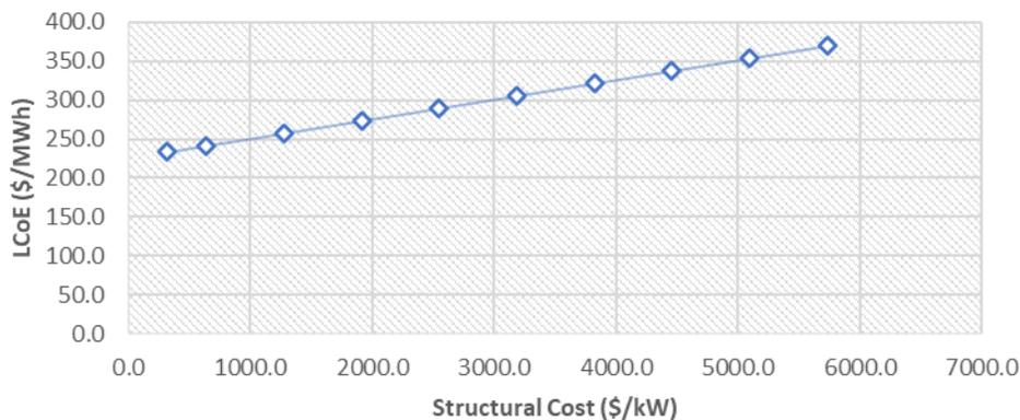
Figure 24 - LCoE vs. Structural Steel Mfg Cost
