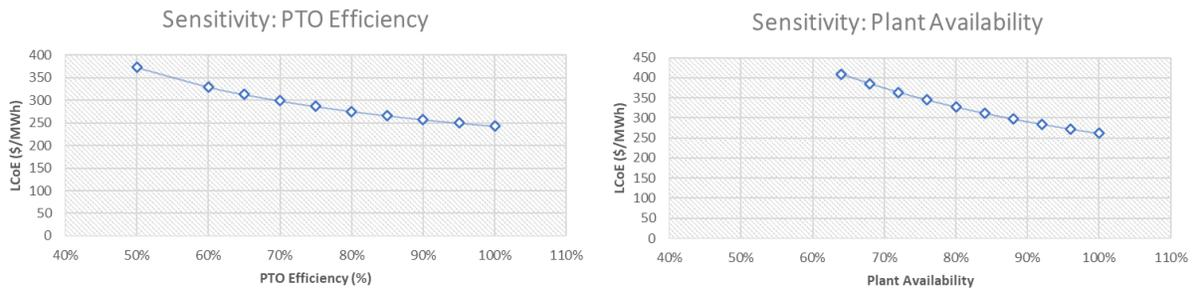
Figure 37 – LCoE Sensitivity to PTO Efficiency and Plant Availability
