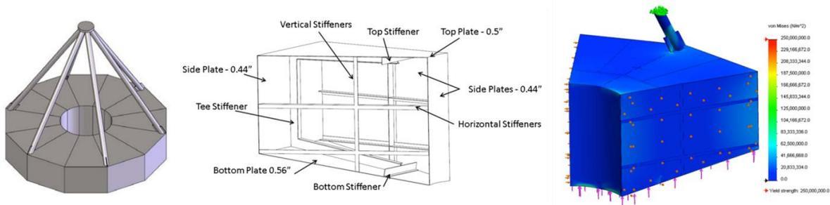
Figure 6 - Structural Design of Absorber buoy
