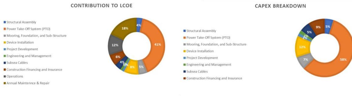
Figure 46 - LCoE and Capex Breakdown of Optimized 100MW Waveswing Plant.
