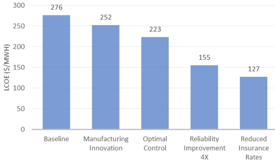
Figure 45 - Cost Reduction Pathway for AWS Waveswing
