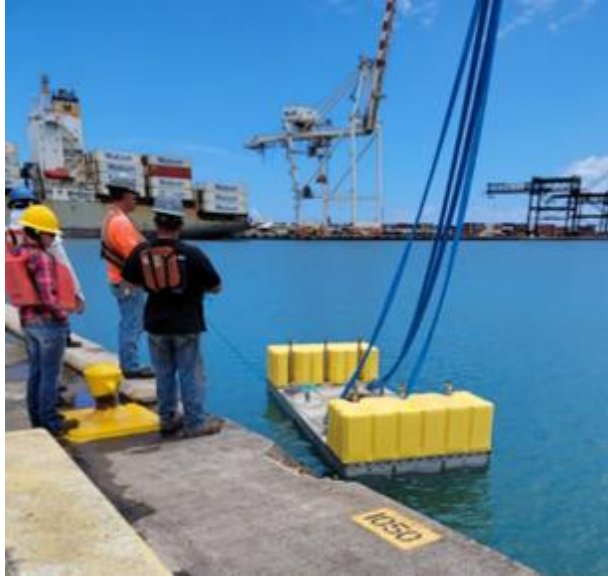
Figure 17 - Heave plate lowered into water for in-harbor operational test
