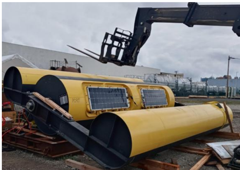
Figure 12 - SeaRAY float assembly.
