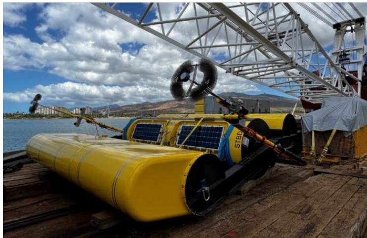
Figure 25 – WPS loaded onto barge.
