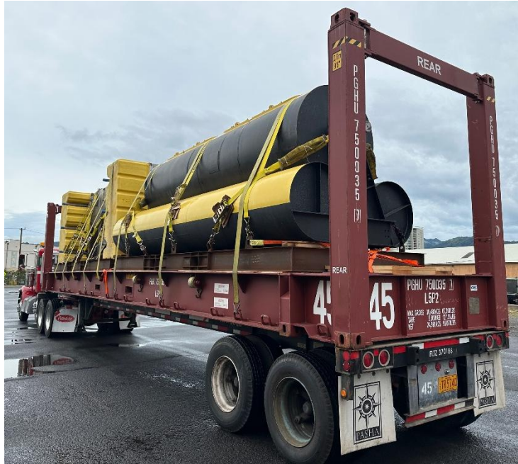
Figure 11 - Heave plate and WPS loaded onto 45' flat rack.
