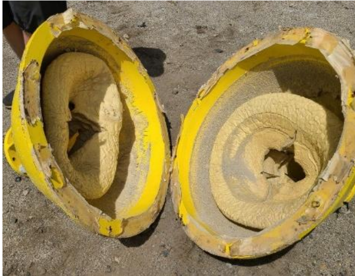
Figure 51 - Collapsed foam inside the mid-column float.
