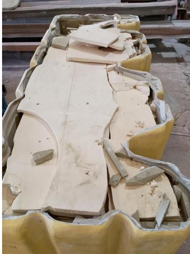
Figure 53 - Foam boards inside heave plate float.
