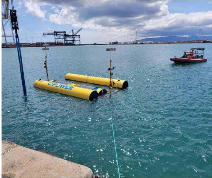
Figure 21 - SeaRAY upright in the water after heave plate flooded to operational position.
