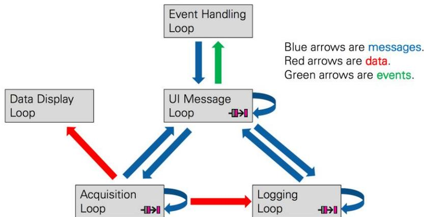
The MOIS software project is a complete application with based on the QMH architecture. The software has three message handlers (MHL): the primary MHL, an acquisition MHL, and a logging MHL.
