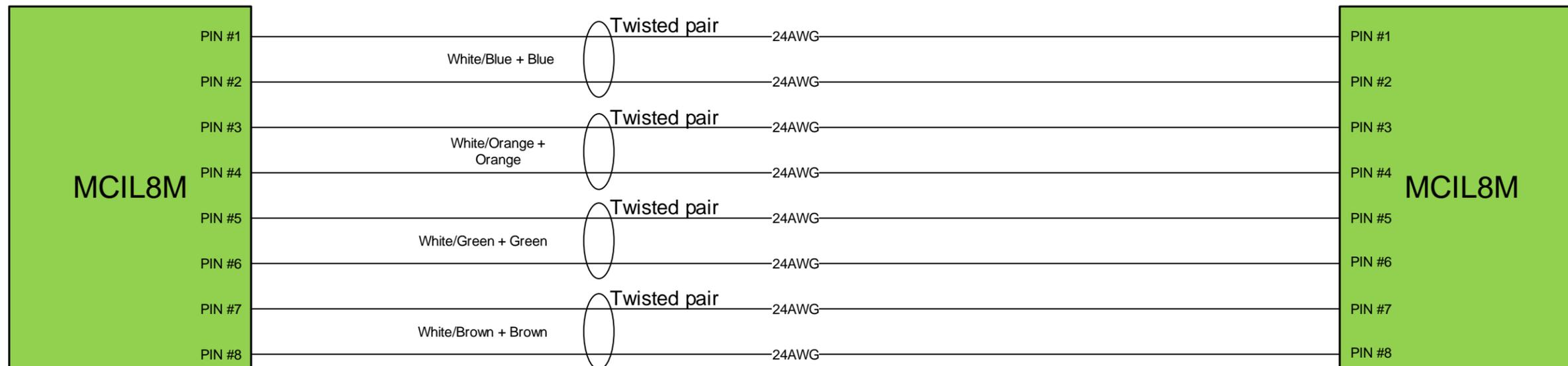
Subconn Power / Ethernet Cable, Type D/P-P4TP24#/4C18# OR equivalent without the power conductors
