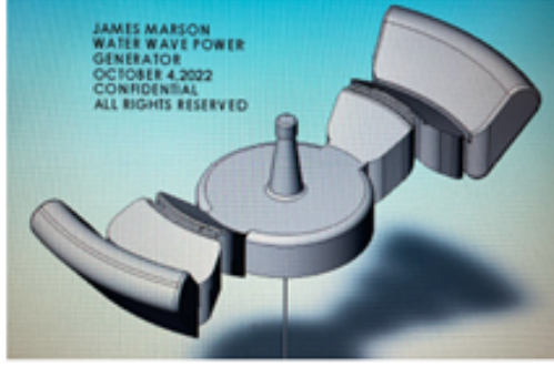
Figure 1: A rendering of one possible device configuration. The device can vary from a circular cross section to this nearly-linear attenuator by varying the number, size, and layout of float sections. Power is extracted through the relative pitching motion between float sections. Optimizing the number, layout, and size of radial and azimuthal sections was a key objective of this work. The work can model affixing the device to an existing floating or fixed structure by considering the inner-most float as connected to this structure.
