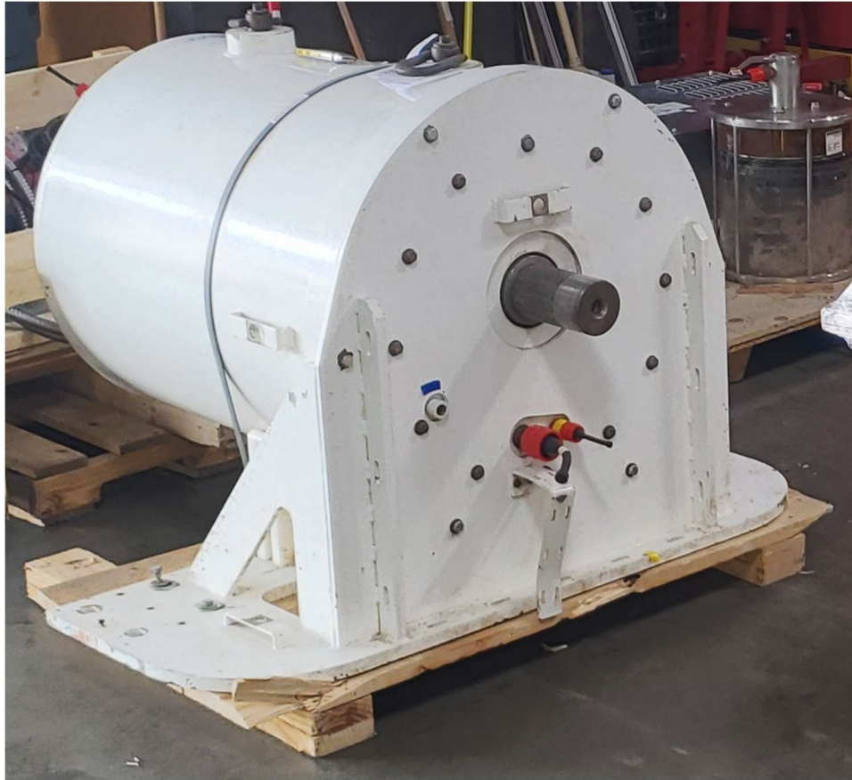
Figure 2 Picture of the submersible housing for the EMF generator that was tested on the dynamometer.
