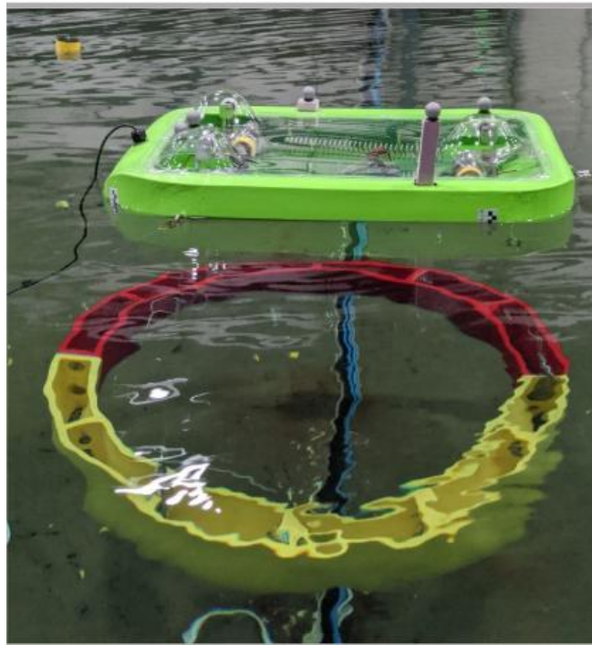
Figure D2b. The 1:50 physical model with transparent lid and submerged reaction ring. Source Figure 16 in the additional notes.
