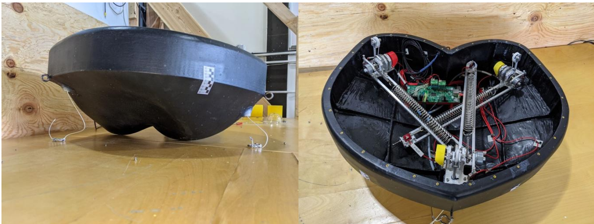
Figure 2. Candidate hull used in the completed-work summary: exterior geometry (left) and internal PTO/sensor arrangement (right). Adapted from source Figure 17.
